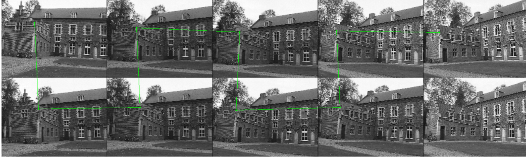
Figure 3.20: One feature detected and tracked over nine images
