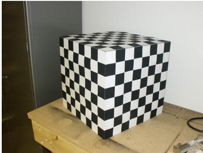
Figure 3.25: Calibration object with known geometry and a checker pattern on all sides (Images courtesy of Stefano Soatto – UCLA. Reproduced from [MSKS03])
