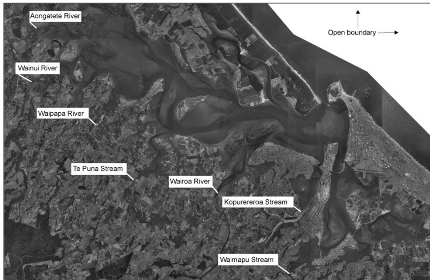
Figure 3.3 Location of inflow boundaries (Wairoa River, Waipapa River, Waimapu Stream, Kopurereroa Stream, Te Puna Stream, Wainui River and Aongatete River) and open boundary for the southern basin of Tauranga Harbour model.
