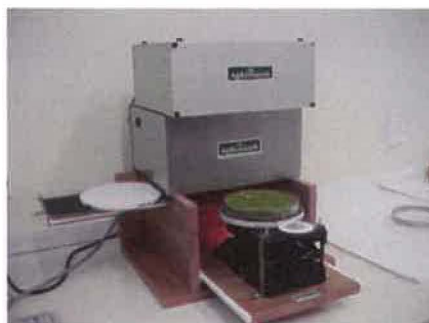
Figure 4.3: Processed sample presented to the NIR instrument.
