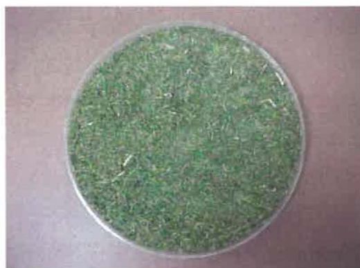
Figure 3.8: Resulting 'shattered' (effectively finely chopped) wet plant sample in a Petri dish.
