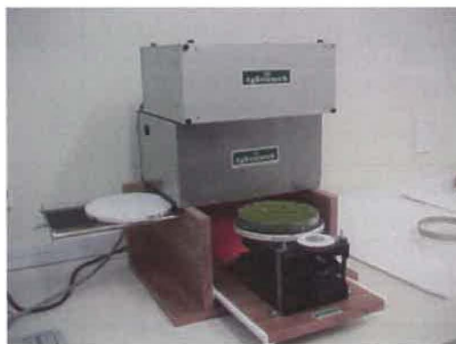
Figure 3.9: Processed sample about to be presented to the KESNIR series 01 instrument with sample presentation unit 1 (SPU1). Also visible is the calibration tile on the left-hand side of the photo. The sample or calibration tile can be slid into the light path and scans taken as required.
