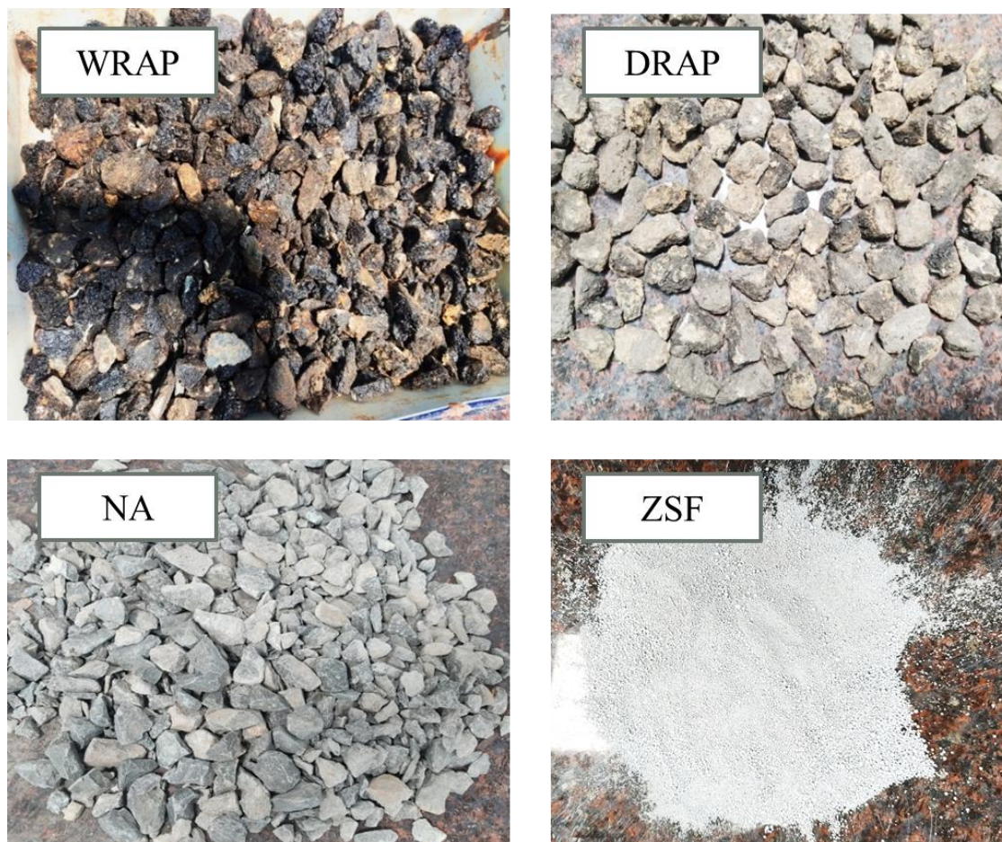
Figure 2. Collection of DRAP, WRAP, NA aggregates and ZSF admixtures used in the present study.
