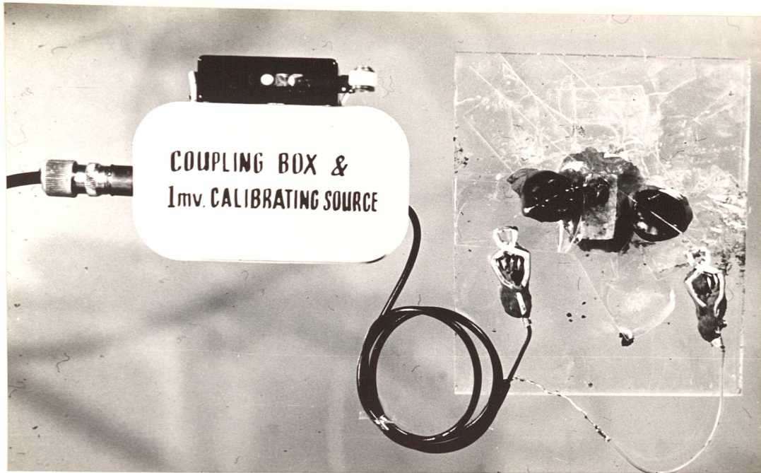
Plate 6.3 The antennal preparation and electrical connection to the coupling box and 1 mV calibrating source. The glass capillaries filled with saline were held on Picien wax mounted on plasticine. The beetle was held in a cork cavity with 'Sellotape'.
