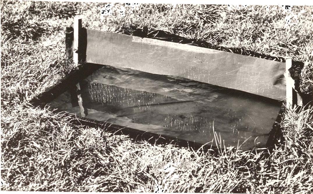
Plate 7.5 The type of trap used in mass trapping trials with Durez paste. The paste (50-150 mg) was applied across the top of the baffle each evening prior to beetle flights.
