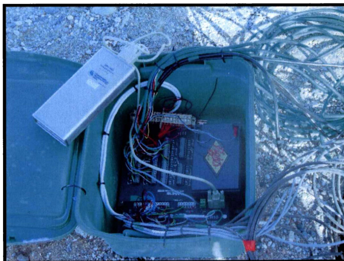
Figure 3.3: TDR probes connected to CR10X datalogger and AM416 multiplexer located in a plastic enclosure on the ground, with SM 192 Storage Module.
