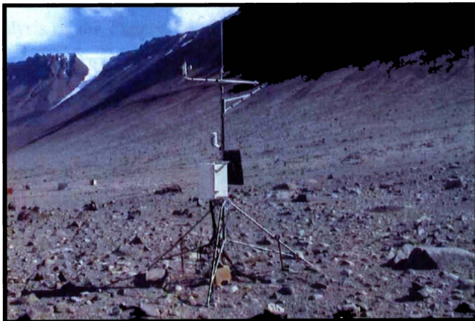
Figure 3.4: Soil climate station at Bull Pass with the CR10X datalogger and AM416 multiplexer located in the enclosure on the A-frame.
