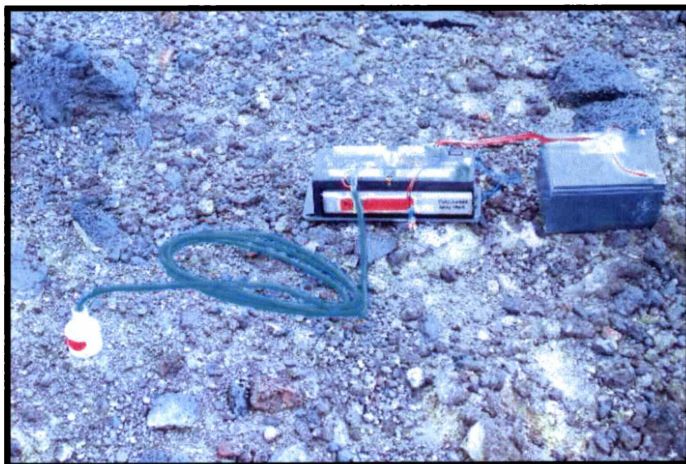
Figure 3.2: Single TDR probe connected to CR10X datalogger.
