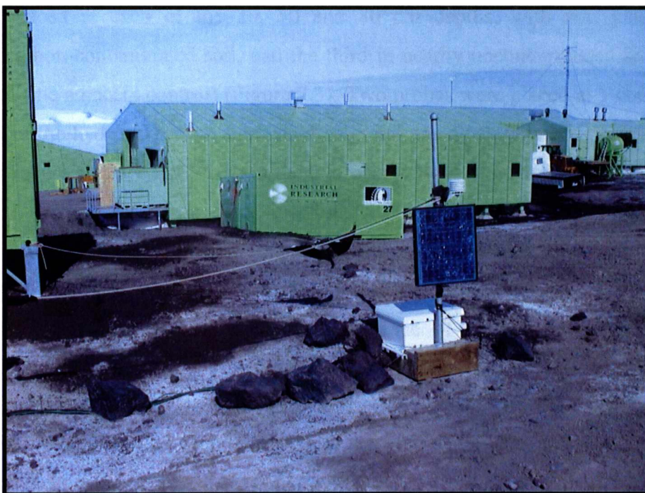
Figure 7.1: Scott Base hydrocarbon-contaminated soil climate station. (Photo courtesy of Ron Paetzold)
