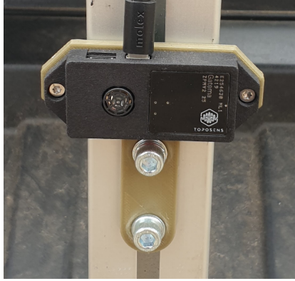
Figure 3.7: Prototype TS3 ultrasonic sensor.
