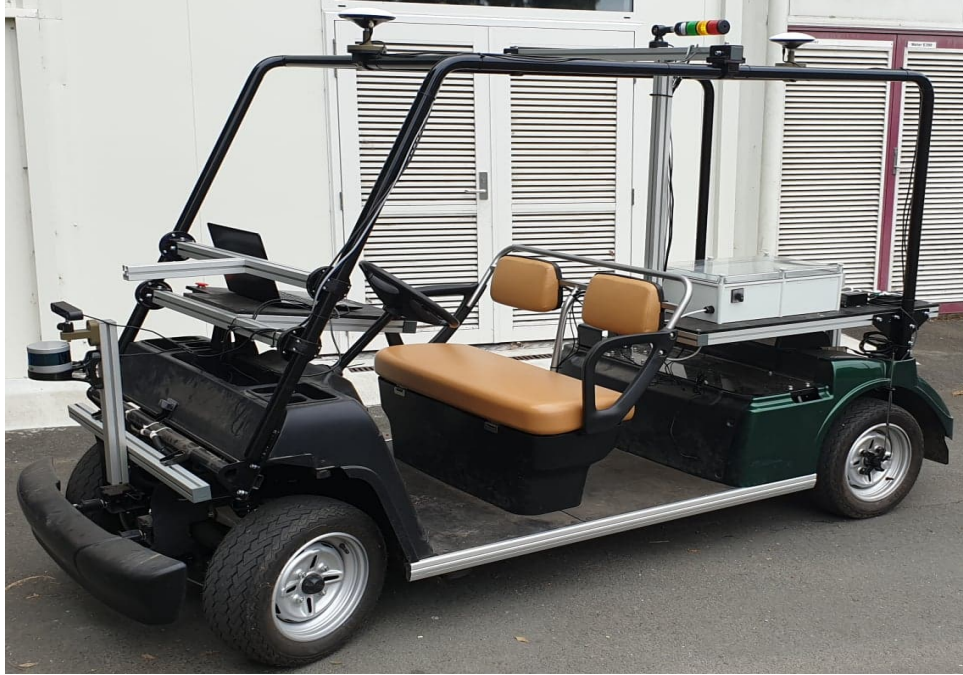
Figure 3.2: Yamaha G30Es golf cart after modifications for autonomous driving.
