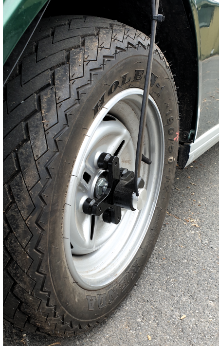
Figure 3.9: Wheel encoder mounted.
