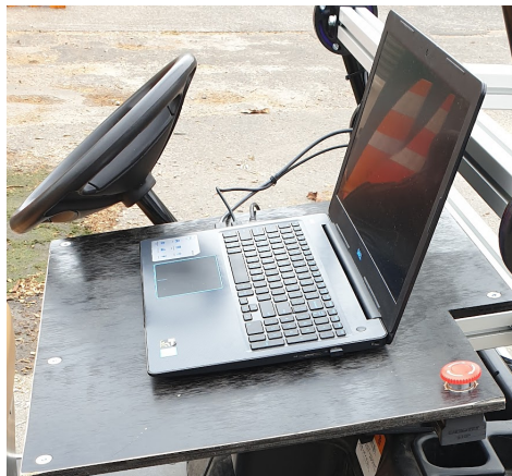
Figure 3.4: Developer station with emergency stop button within reach.
