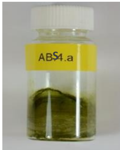
Figure 2.3. Crude extract preparation as exemplified by ABS4a (first 2 g extraction of Splachnidium rugosum collected in summer). This includes a) homogenisation, b-c) filtration and transferal to flask, d-e) evaporation of solvent, and f) resultant extract in scintillation vial.
