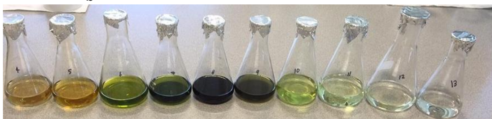
Figure 3.5. Separation of 20g extract of ABS9a by reversed phase C_{18} column chromatography. This includes a) elution of early polar fractions with a distinctive green colour, b) elution of fractions in the non-polar region, and c) collection of all fractions produced from the C_{18} column.
