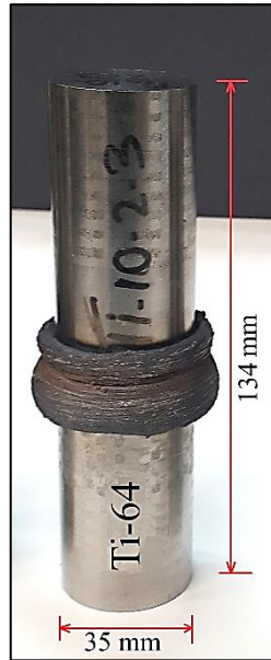
Figure 49: Image shows RFW joint between Ti-64 and Ti-1023.
