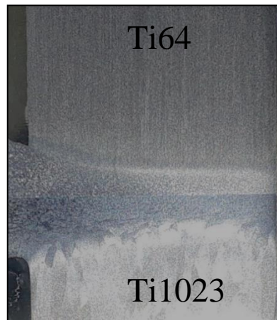
Figure 51: Image of macro specimen for RFW joint between Ti64 and Ti-1023.
