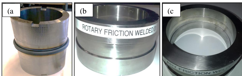
Figure 28: Image displays (a) key-way slots, (b) as welded joint after proof machining and (c) top view of RFW joint between S355J2 and SS316L.
