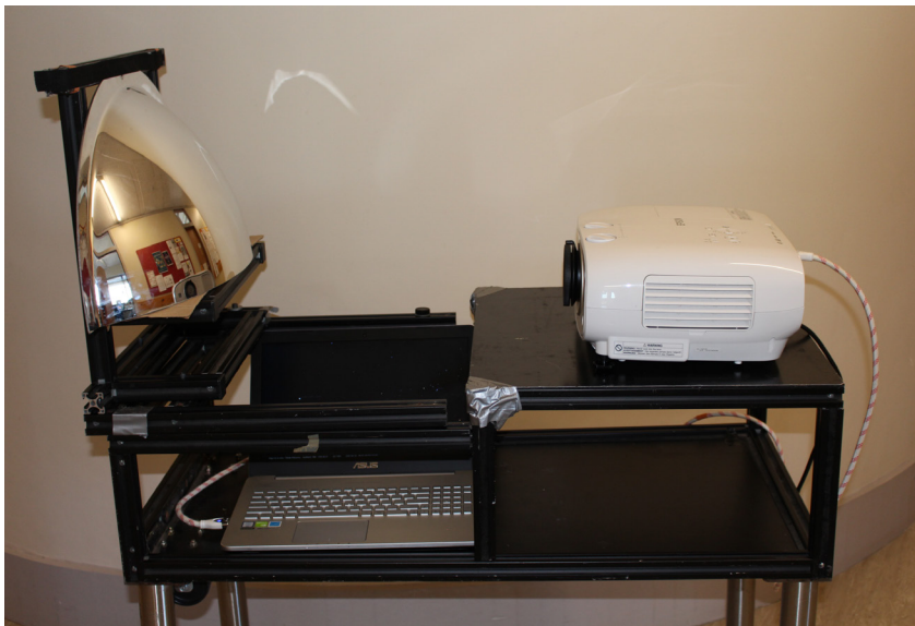
Figure 2: Planetarium Dome equipment setup for inside the dome, from left to right mirror, computer and projector.
