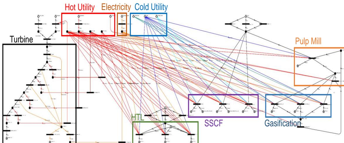
Figure 2: Maximal structure of the P-graph for the biorefinery processing of forest biomass residues.
