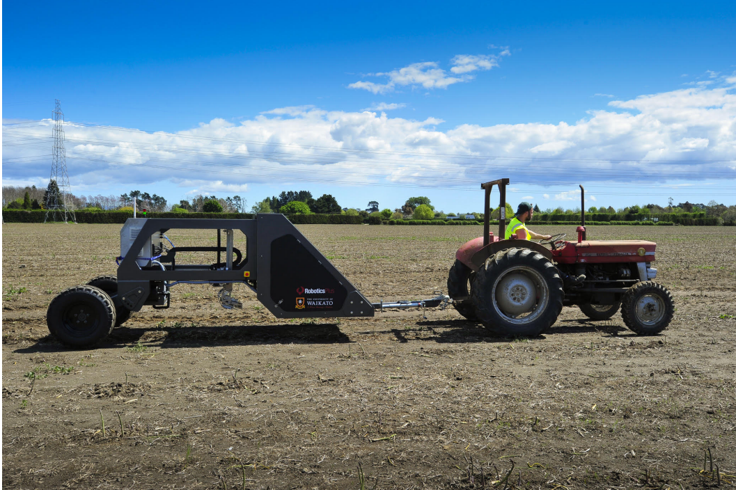
Figure 5.4: AHR-2 operating on a New Zealand asparagus row.
