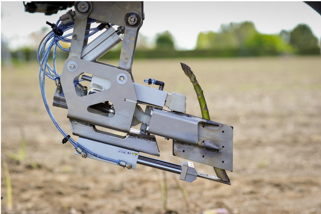
Figure 5.8: AHR-2's end-effector. Gripping and cutting actions can be individually actuated via pneumatics.
