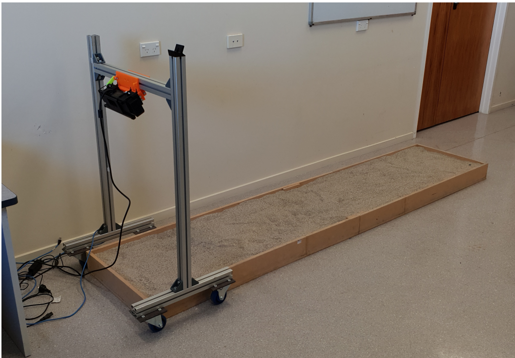
Figure 3.3: Mockup asparagus bed. Frame is constructed from MDF and Kinect mount is constructed from 3D printed PLA.
