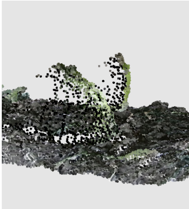
Figure 3.7: Pointcloud of two spears demonstrating a number of flying pixels. These pixels extend far behind the imaged spear in the direction of the camera's optical axis.
