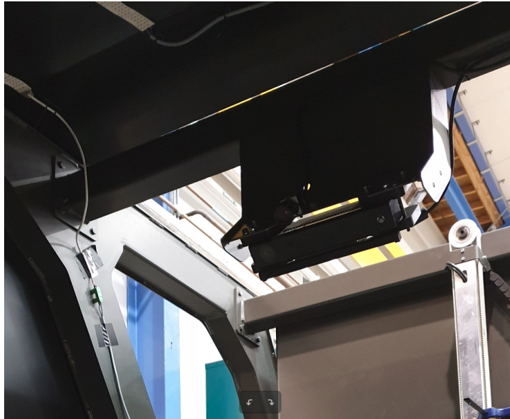
Figure 4.5: AHR-1's camera mount with Microsoft Kinect V2 and Basler ACE cameras attached.
