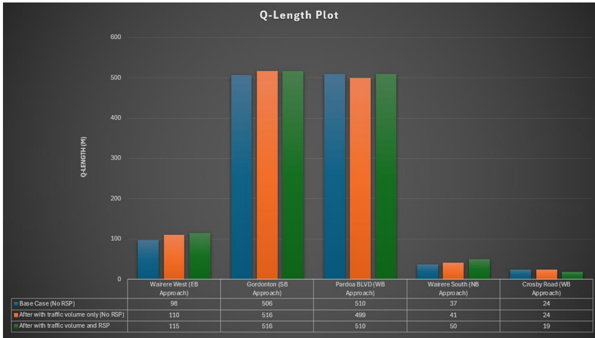
Figure 45. Vehicle Max Queue Length plot for Wairere Drive and Resolution Drive Roundabout
