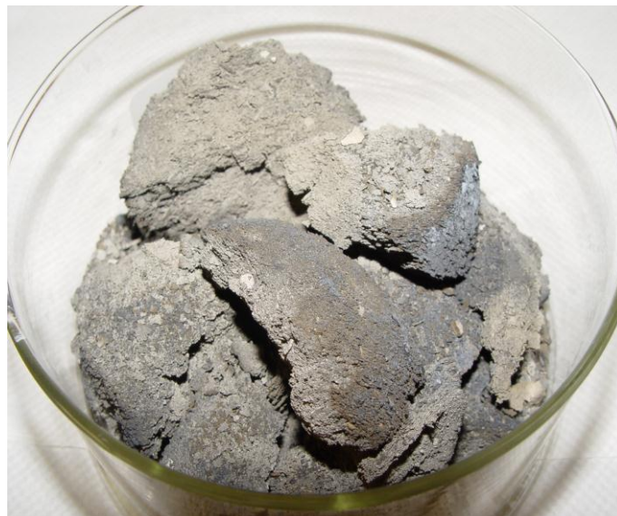
Figure 4.23: Macrograph of the combustion reacted powder A (produced from 500 g of as-milled powder with DPR 22:1) before ball milling
