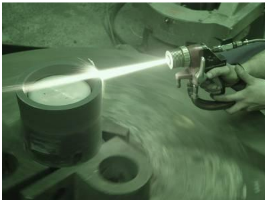
Figure 3.3: HVOF thermal spraying of composite powder feedstock
