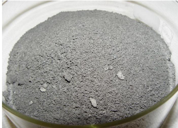
Figure 4.31: Macrograph of the combustion reacted powder B (produced from 500 g of as-milled powder with DPR 13.2:1) before ball milling
