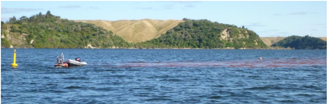
Figure 19. Dye plume produced on the lake surface. Mixing device and dye metering equipment on the left with a surface plume visible moving towards the right (north).
