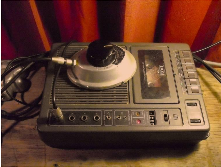
Figure 18: Larsen-Jensen's 'pie-dish' oscillator used with tape-machine amplifier (Reprinted with permission from Felix Larsen-Jensen, 2012).
