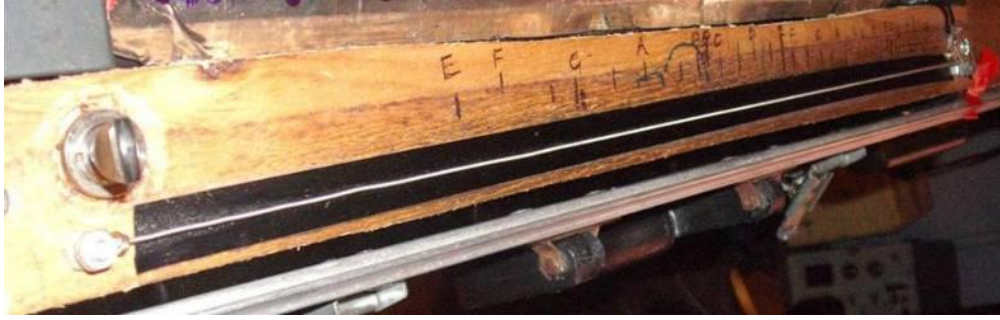
Figure 22: The 'ribbon controller' method of controlling the oscillator (image by author, 2013).
