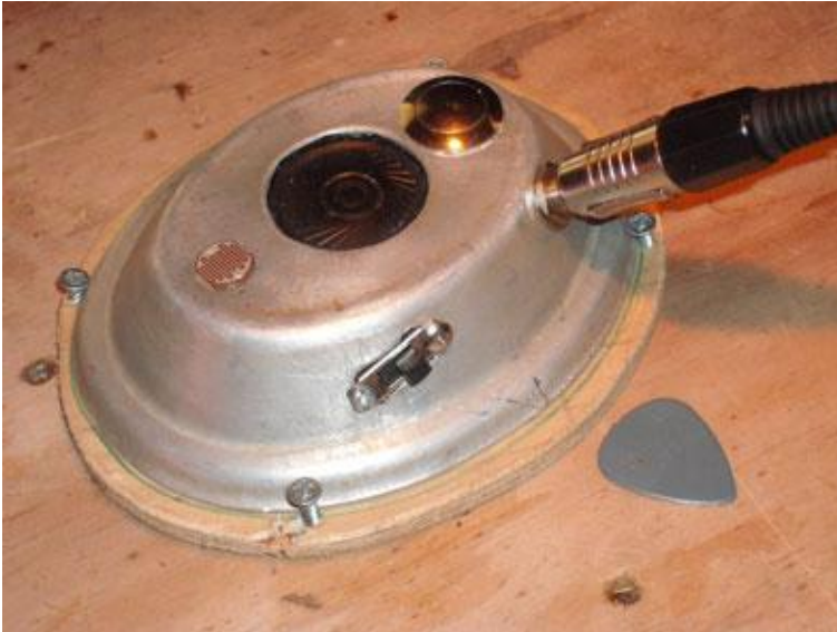
Figure 21: Light dependant Oscillator (Reprinted with permission from Felix Larsen-Jensen, 2011).
