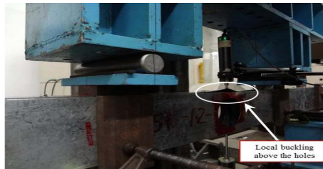
Figure 2-3: Four-point bending test with experimental and numerical analysis [22].
