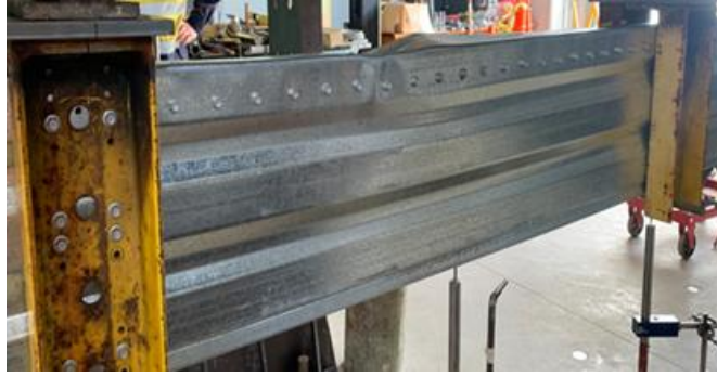
Figure 2-6: Four-point bending test [7].
