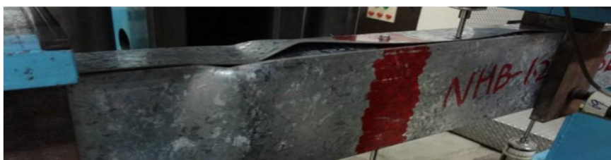
Figure 2-4: Four-point bending test with experimental and numerical analysis on the built-up beam [24].
