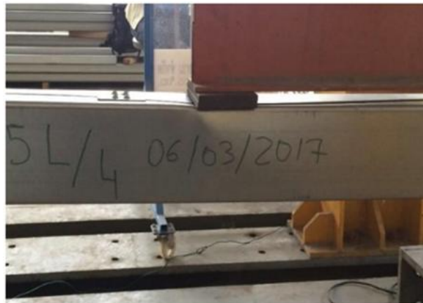
Figure 2-2: Four-point bending test on built-up beam [21].
