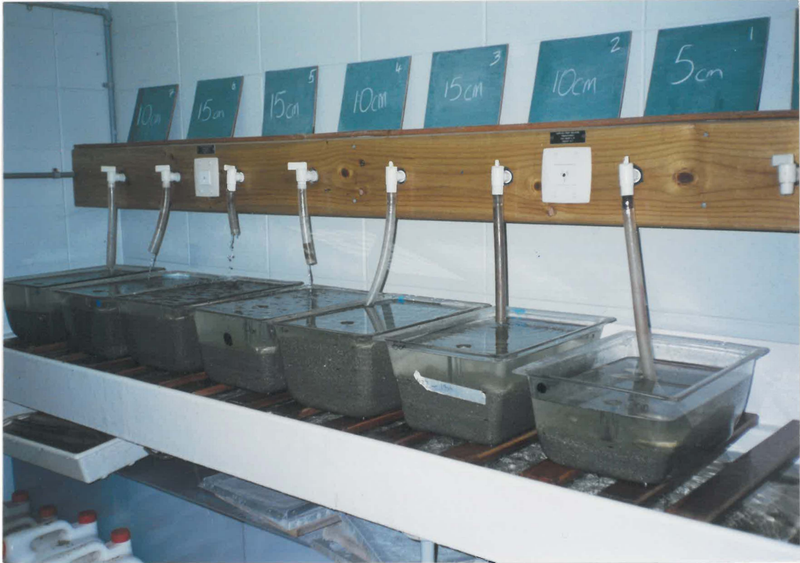
Plate 5.4 The arrangement of experimental aquaria in the tankroom at the University of Waikato salt water circulation room
