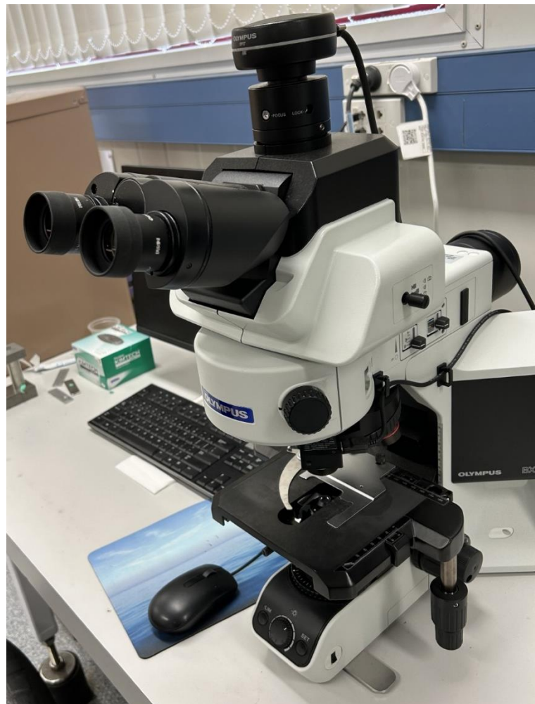
Figure 26: Olympus BX53 optical microscope used for microstructural analysis
