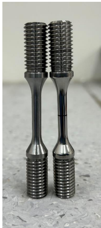
Figure 33: High-cycle fatigue testing samples: original machined sample on the left and the same sample after polishing on the right
