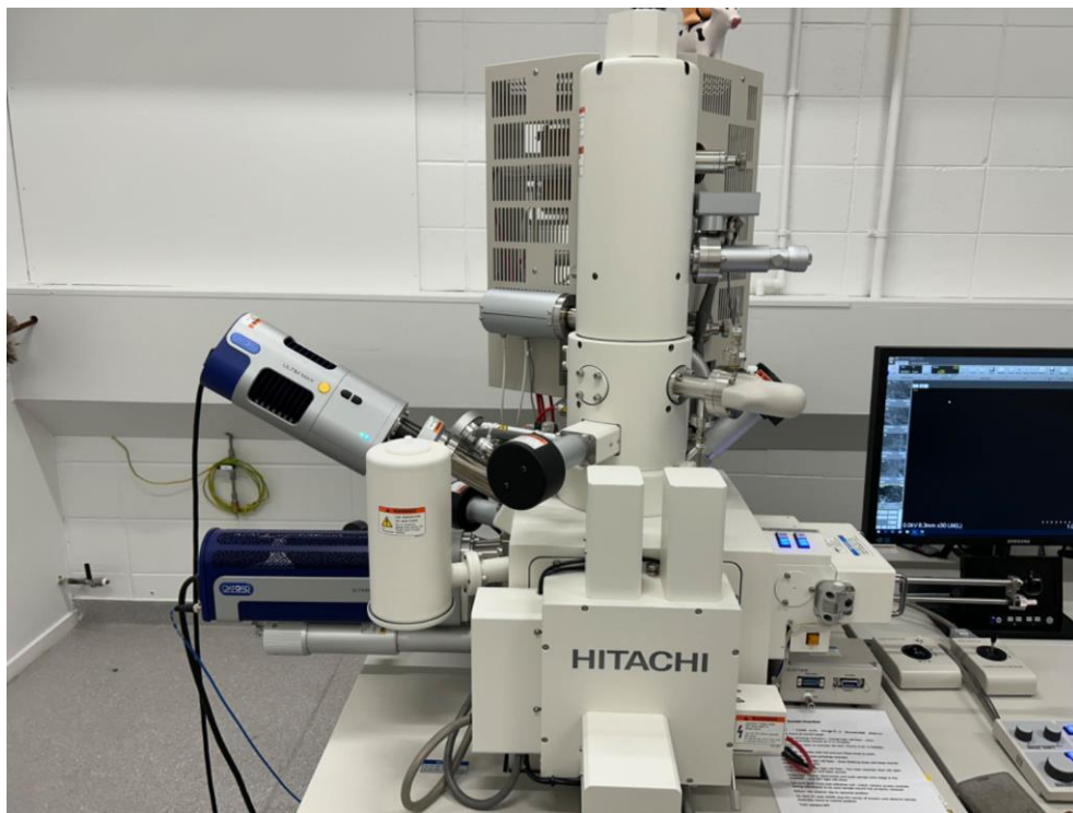
Figure 27: Hitachi S-4700 scanning electron microscope used for detailed microstructural analysis
