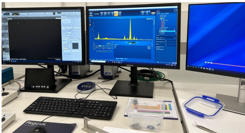
Figure 28: Software interface used for EDS analysis to perform elemental and chemical analysis
