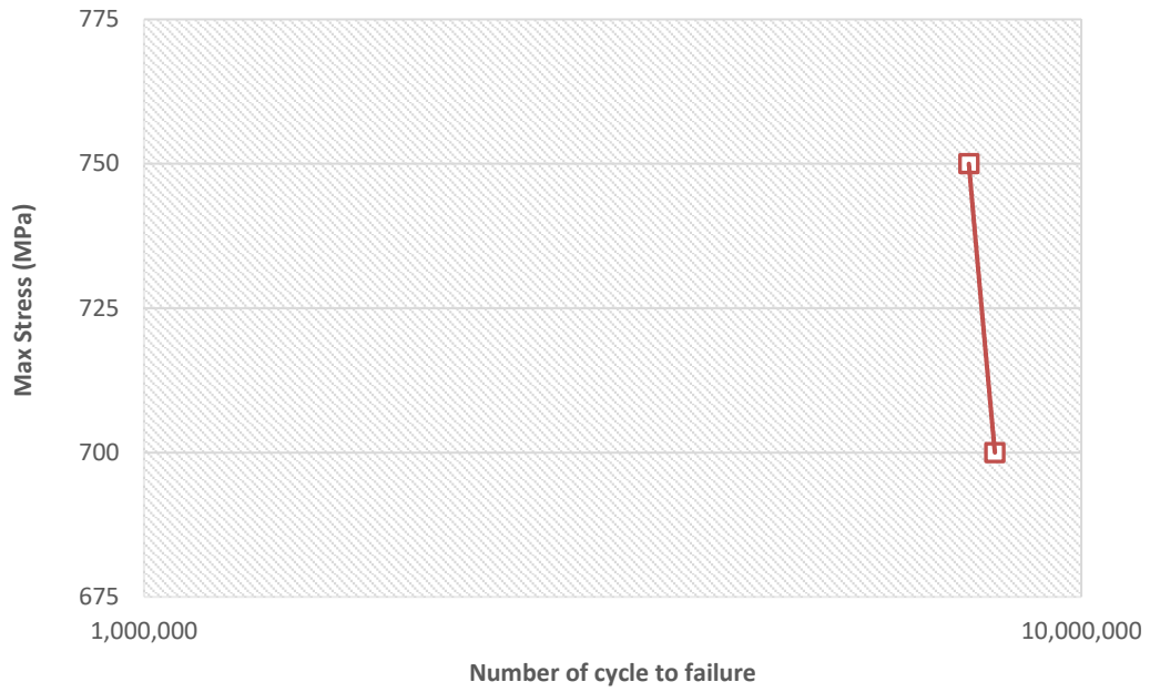
Figure 59: S-N curve for Ti-5553 alloy aged at a 5°C/min heating rate
