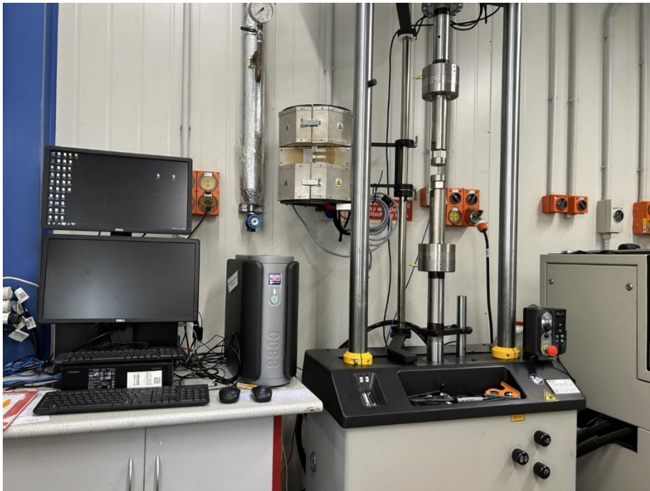
Figure 34: Instron 8801 Servo-hydraulic dynamic testing machine used for fatigue testing
