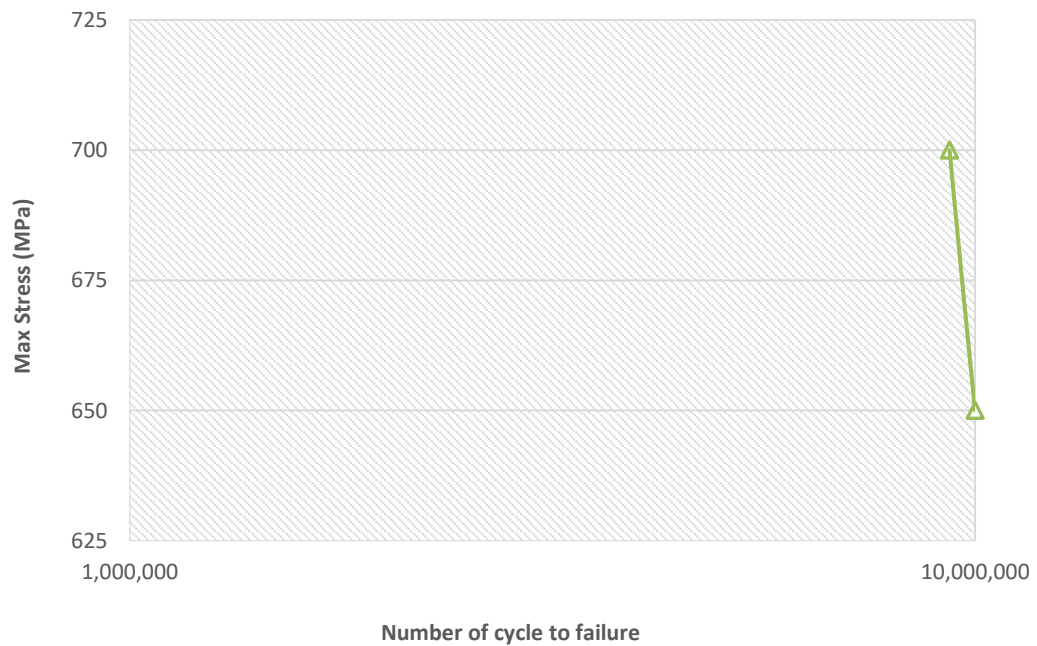
Figure 60: S-N curve for Ti-5553 alloy aged at a 10°C/min heating rate
