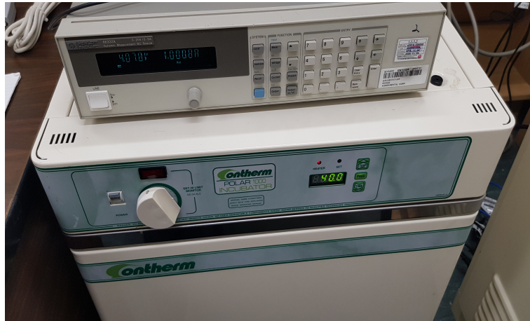
FIGURE 4.4: Experimental setup of the 66332 on top of the Polar 1000 incubator set to 40°C. The 66332 output is on the reverse of the device.
