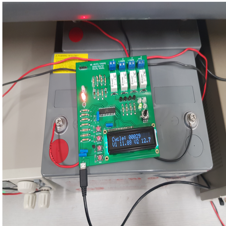
FIGURE 3.12: The first version of the battery cycling board running on a pair of lead-acid batteries
