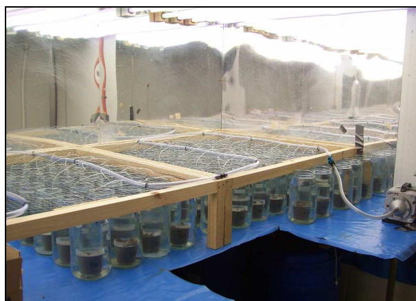
Figure 19: Experimental layout of inoculated jars with lake sediment in the CT room with the aeration frame in place (photograph by Author)
