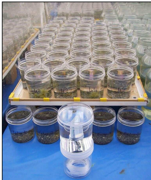
Figure 20: Experimental layout of the treated sieved lake sediment, the 5 extra containers and the container with the temperature and light probe (photograph by Author)
