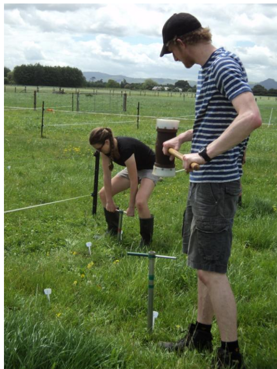
Figure 3.2 Example of soil coring taking place at DairyNZ's Scott Farm, Newstead.
