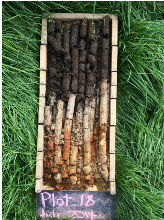
Figure 3.5 Example of 15 cores from plot 18 being laid out on a coring board before being divided into 10cm increments.
