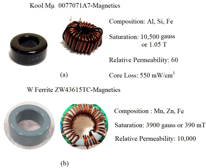
Figure 3.13: Magnetic properties comparison: (a) Kool \mu 0077071A7 powdered-iron toroid; (b) W-Ferrite ZW43615TC toroid [76, 77]
