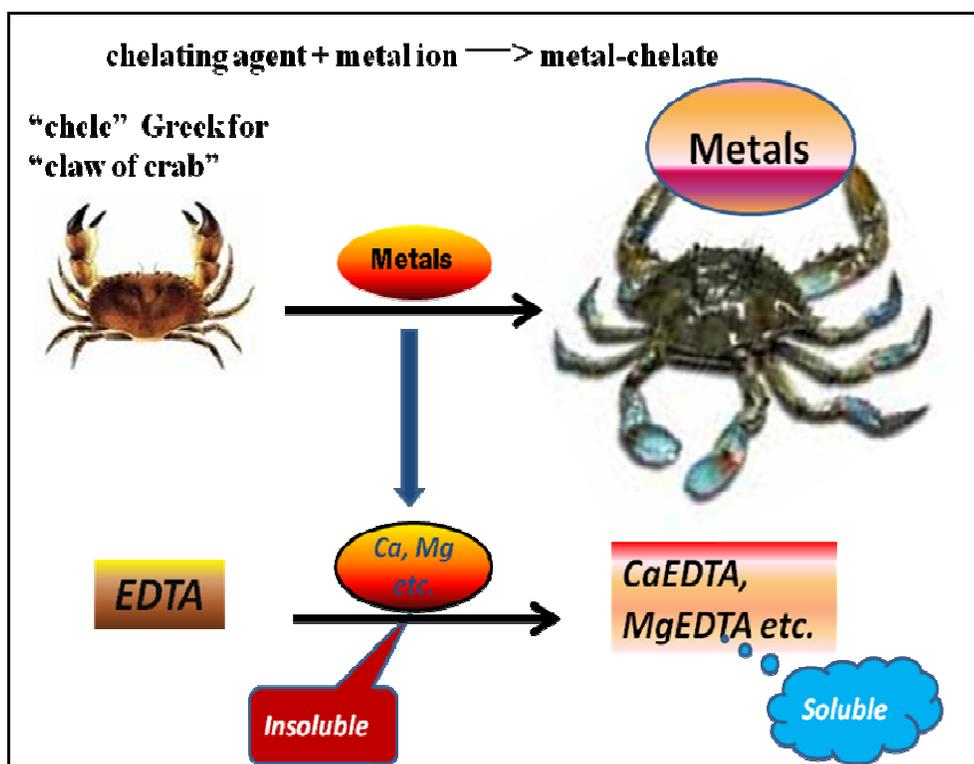
**Figure 1.1** Chelating agents are used for a wide variety of industrial applications to bind undesirable metal ions. For example EDTA is used in the removal of precipitated calcium (Ca) and magnesium (Mg) on the surface of machinery in the cleaning process of dairy manufacturing plants.
