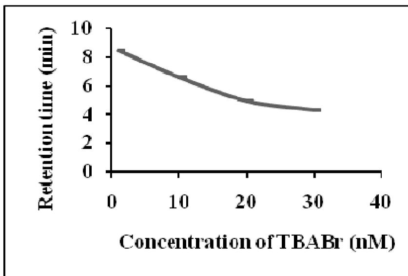
**Figure 3.6** Effects of concentrations of tetrabutylammonium bromide (TBABr) in the mobile phase on the retention of  $[\text{Fe(III)EDTA}]^-$  during chromatographic separation when other parameters remain the same.
