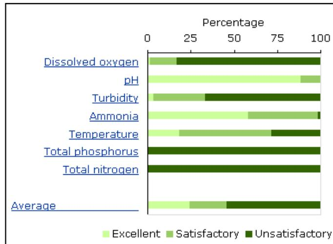
**Figure 5.21** Water quality, as determined by the percentage of samples rated as excellent, satisfactory, or unsatisfactory against accepted ecological standards, of routinely monitored factors in the Waitoa River at Mellon Road..
