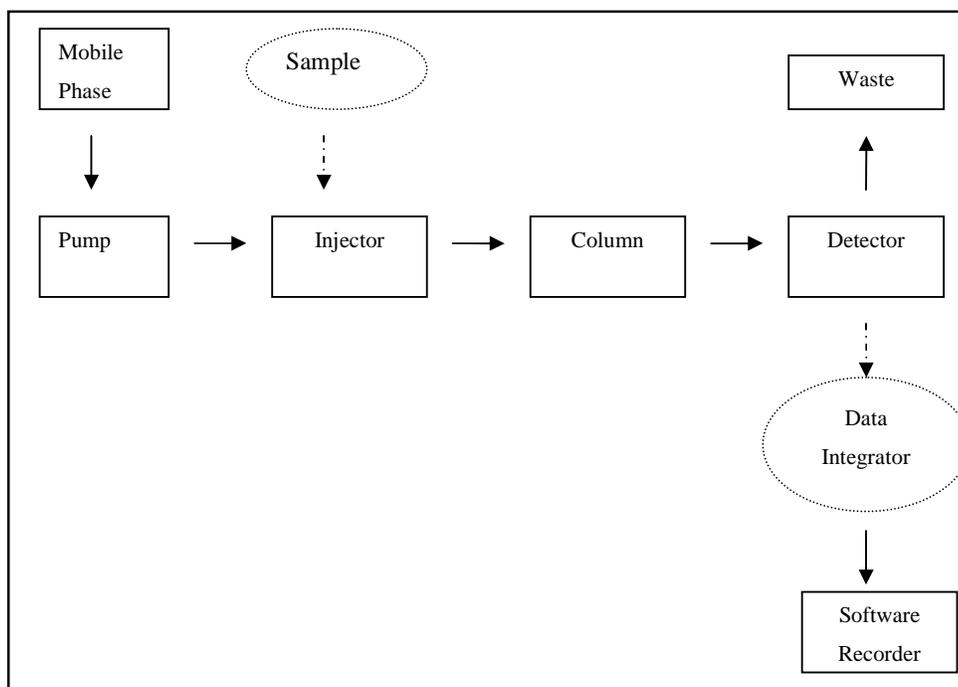
**Figure 3.2** HPLC System Components for the determination of EDTA applied in this research.
