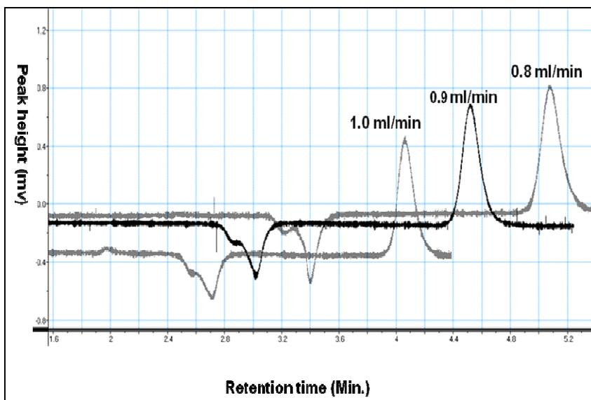
**Figure 3.7** [Fe(III)EDTA]<sup>-</sup> is retained longer with a lower flow rate of the mobile phase during chromatographic separation when other parameters remain the same.
