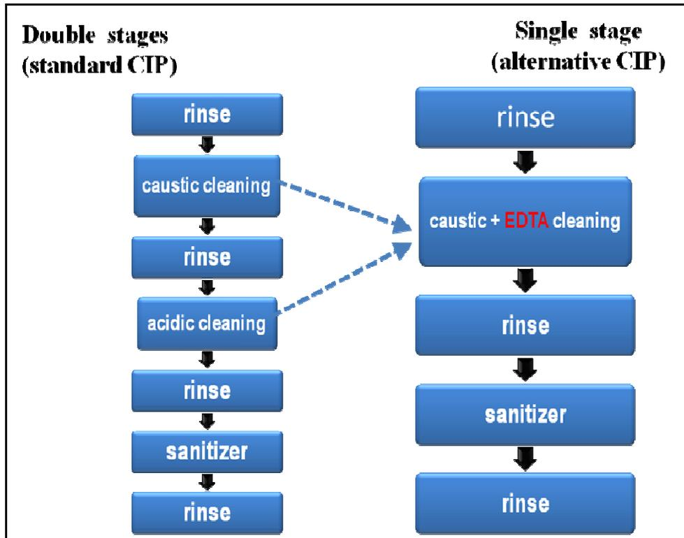
**Figure 1.2** A comparison of a standard two-stage, and the alternative using EDTA as a one-stage cleaning procedure of the CIP system applied in manufacturing plants in the New Zealand dairy industry.
