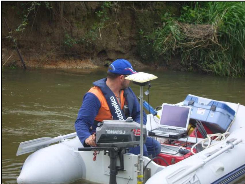
**Figure 6.9** Collecting bathymetric data using an echosounder on a survey vessel for the purpose of hydrodynamic modelling within the Waitoia River.
