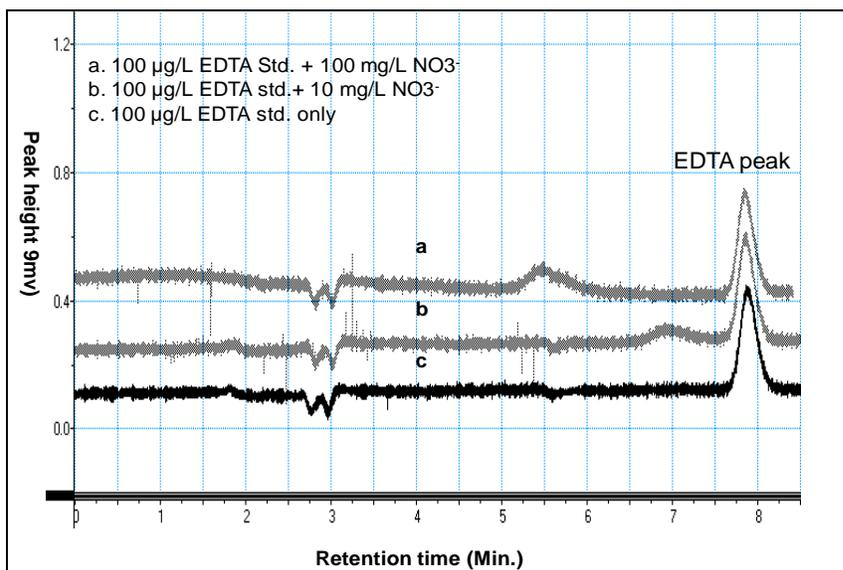
Figure 3.10 The effect of addition of nitrate on HPLC analysis of EDTA.
