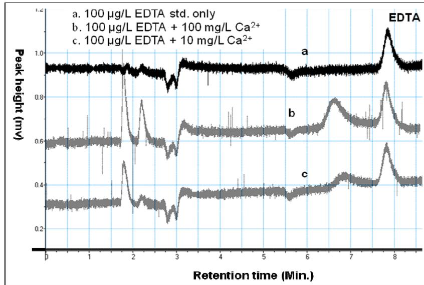
Figure 3.11 The effect of addition of calcium on HPLC analysis of EDTA.
