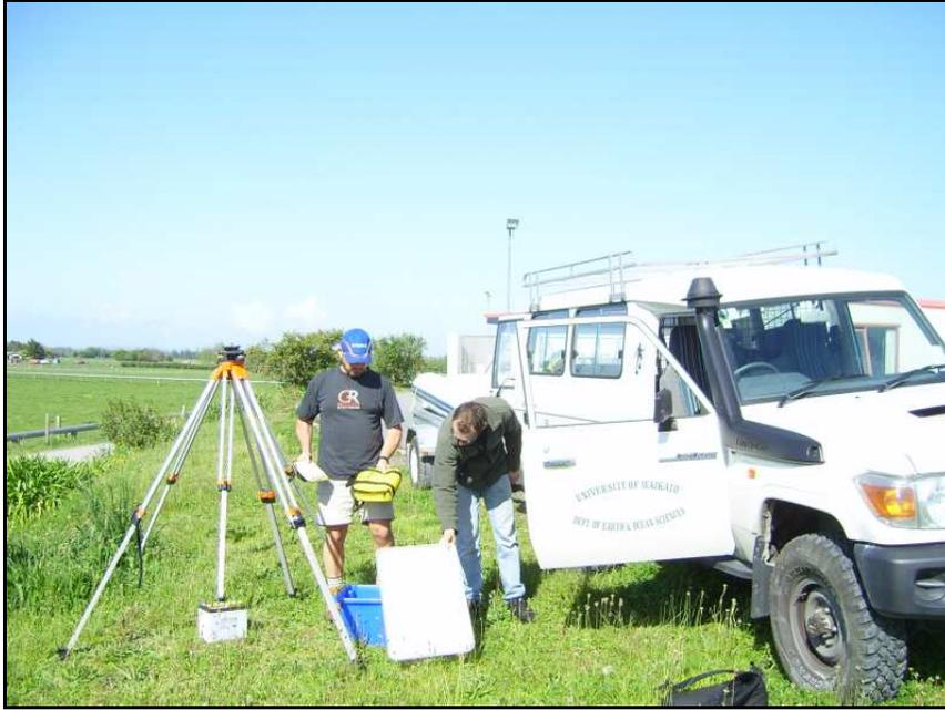
**Figure 6.8** Setting up a standard GPS station for a known point before the collection of bathymetric data for the Waitoia River.
