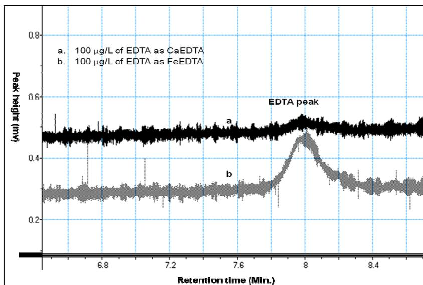
**Figure 3.15** Absorbance comparison of 100 µg/L EDTA as  $[\text{Fe(III)EDTA}]^{-}$  and  $[\text{Ca(II)EDTA}]^{2-}$ .
