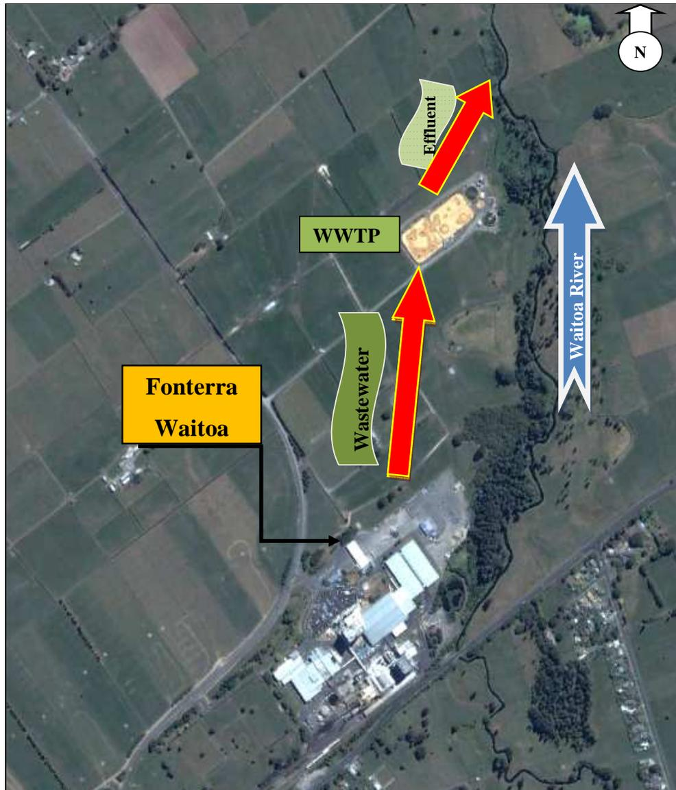
*Figure 1.4 Dairy effluent discharges into the adjacent waterway of the Waitoa River after treatment at the Fonterra Waitoa dairy site, New Zealand. WWTP is the wastewater treatment plant.*
