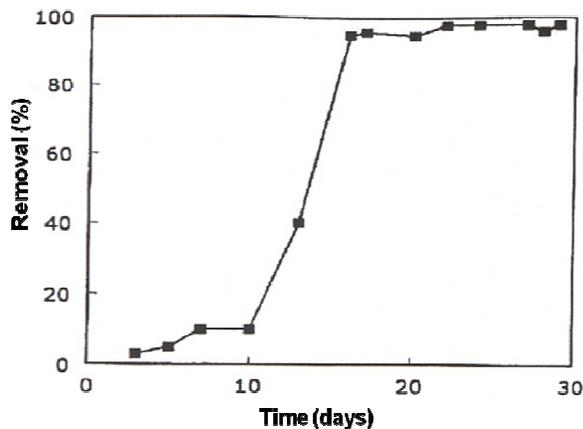
**Figure 2.5** EDTA removal efficiency of dairy wastewater associated with the sludge retention time at pH value of 8.7 - 8.9
