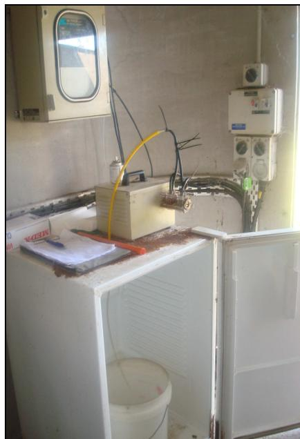
**Figure 4.10** A 24-hour composite flow-proportional sample collection setting of wastewater from the cheese drain, wet process plant, influent, and effluent at the Waitoa dairy site, Fonterra Co-operative Group Limited.
