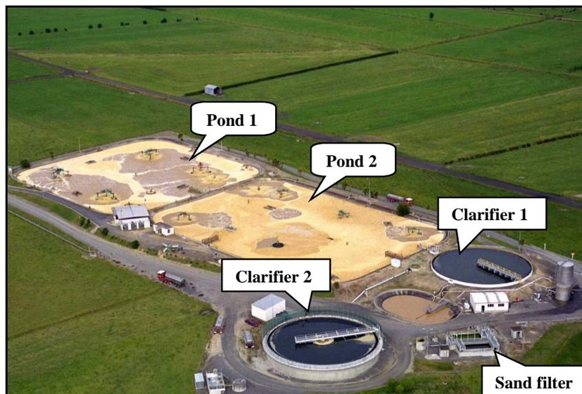
**Figure 4.3** A layout of the wastewater treatment plant at the Waitoa dairy site.
