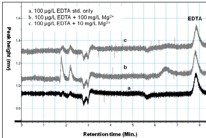
Figure 3.12 The effect of addition of magnesium on HPLC analysis of EDTA.
