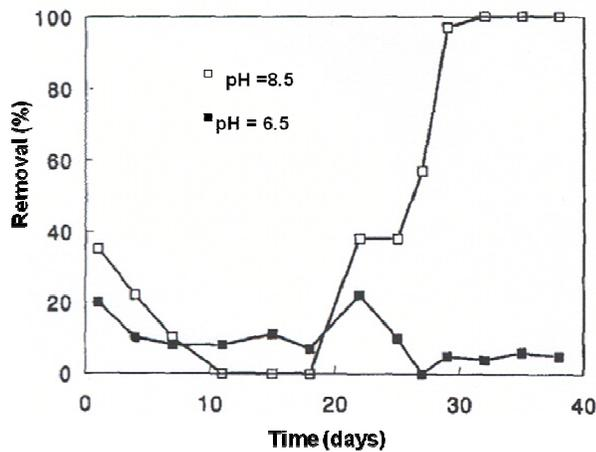
**Figure 2.4** EDTA Removal efficiency of dairy wastewater at pH 6.5 ■ and 8.5 □.
