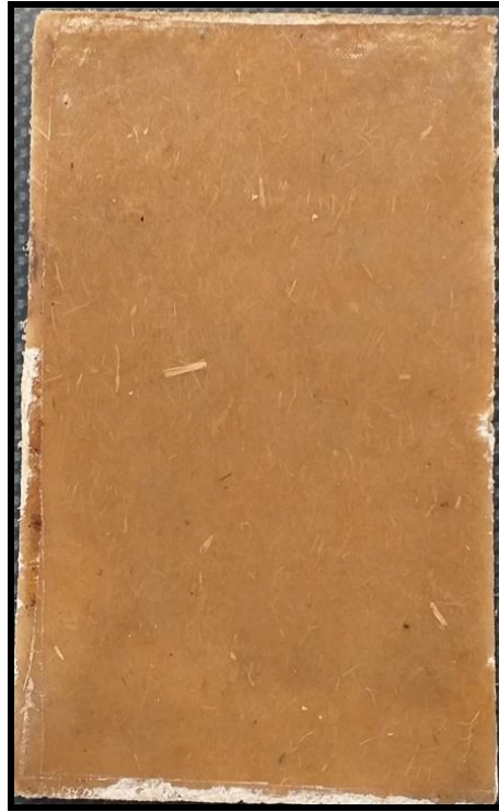
Figure 5.3: Hemp composites with 30 wt% fibre content fabricated by compression moulding.
