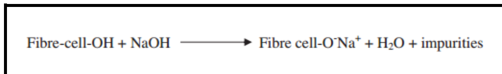
Figure 2.16: Chemical reaction between fibre cell and NaOH [29].
