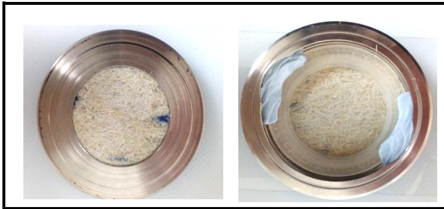
Figure 4.3: Photographs of a sample prepared for XRD analysis. Note the following: top view (left) and bottom view (right).
