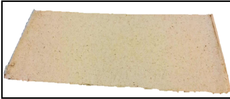
Figure 4.5: A complete hemp fibre mat produced using DSF, (approx. 1000 x 300 x 0.80 mm).
