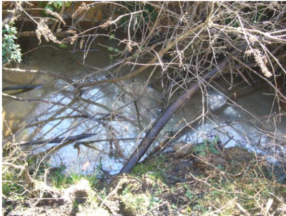
Site 8: Groundwater seepage from hill side, Taeda Road hill top. Sample was taken from a small gully (left) where groundwater seeping from the north-facing slope (right) had ponded. Note oily sheen on the water surface.
