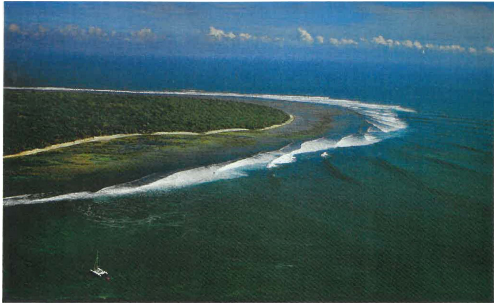
Plate 8.4. Aerial view of an island surfing break, where the wedge (reef edge) is continually bending away from the approaching waves, which compensates for refraction and produces surfable peel angles over a very long distance. Note the region at the top of the photo, where wave peel angles are very low and unsurfable where the island faces the swell direction and waves are closing out. (Photo Dick Hoole – In : Uluwatu. Tadevan Holdings Pty Ltd. 1998)
