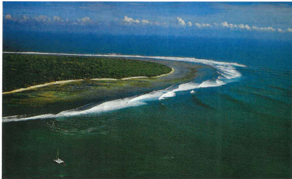
Plate 4.1. Aerial view of an island surfing break, where the wedge (reef edge) is continually bending away from the approaching waves, which compensates for refraction and produces surfable peel angles over a very long distance. Note the region at the top of the photo, where wave peel angles are very low and unsurfable where the island faces the swell direction and waves are closing out. (Photo Dick Hoole – In : Uluwatu. Tadevan Holdings Pty Ltd. 1998)
