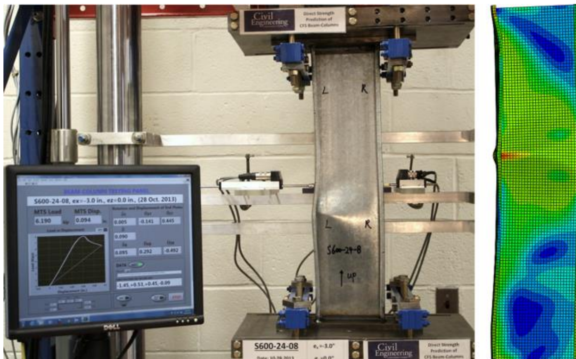
Figure 3.10 Failure mode determined by FE model versus experimental (S600-610-8) (test set-up adopted from [32]).
