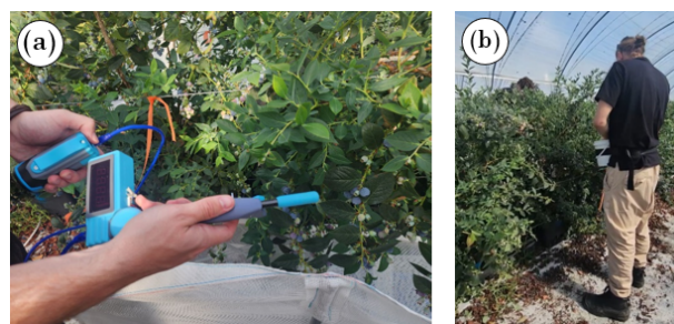
Fig. 2. (a) Hand-held shaker developed by the University of Waikato shaking a cluster of Masena blueberries; (b) Traditional hand-harvesting method where workers place blueberries into a waist-strapped bucket.
