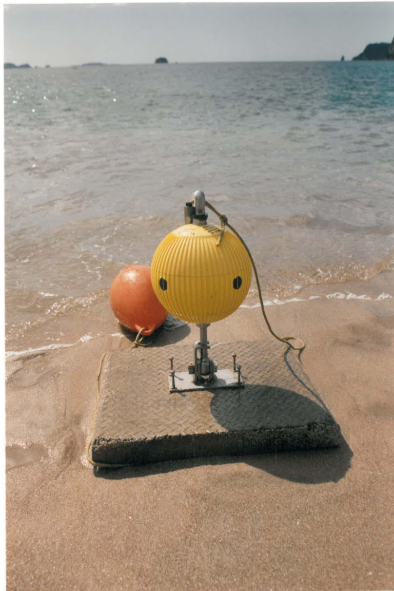
Fig. 6.2 The S4 current meter
