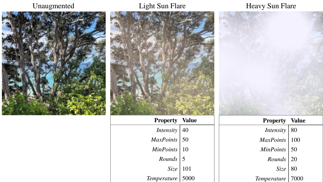
Figure 4.4 Comparison of unaugmented input image (left) to output sun flared images (centre, right)
