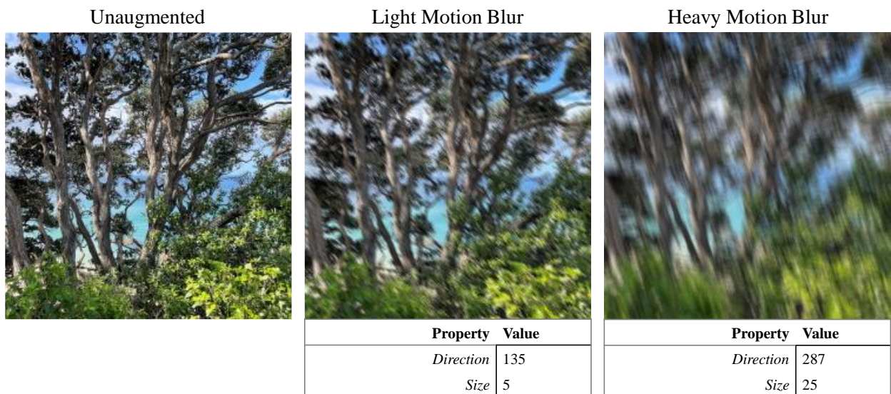
Figure 4.2 Comparison of unaugmented input image (left) to output motion-blurred images (centre, right)
