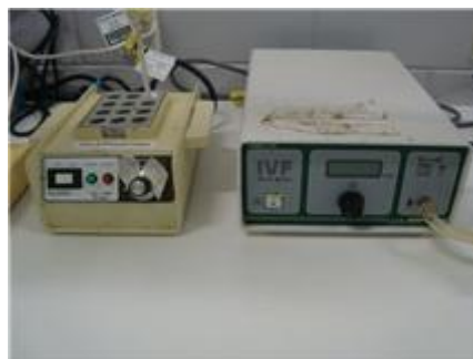
Figure (2.1): Aspiration machine and tube warmer machine. Aspiration device was set on -40 to -45 mmHg and tube warmer was sat on 28°C.
