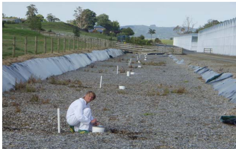
Fig. 1.1 Gas sampling by Sören at a large denitrification bed receiving effluent from a glasshouse in Karaka (NZ)
