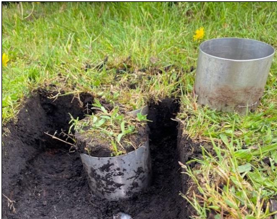
Figure 3.10 Example of soil cores collected in field (Photo credit: David Campbell, 2021)
