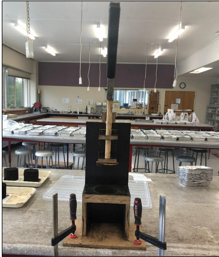
Figure 3.12 Device used to remove soil cores from the steel rings
