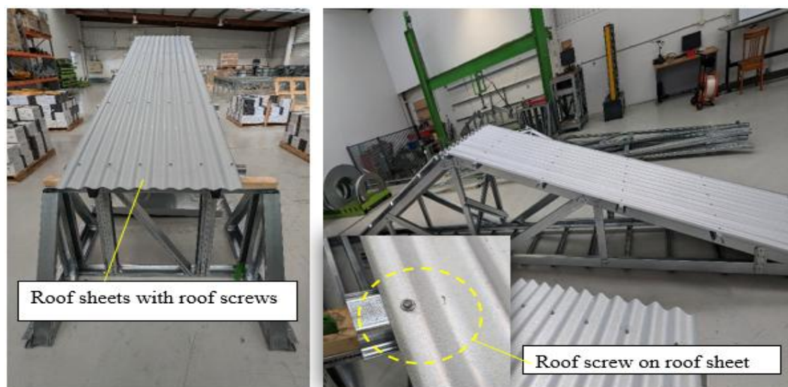
Figure 3-12: Roof sheets and roof screws on truss experiment
