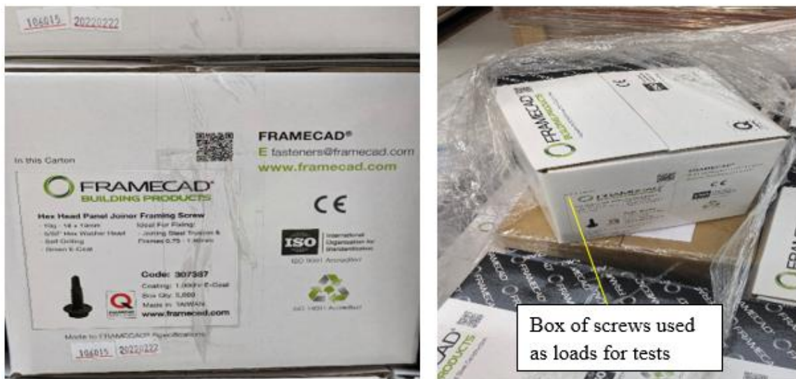
Figure 3-32: 15.75kg box of screws which are applied as loads during the tests
