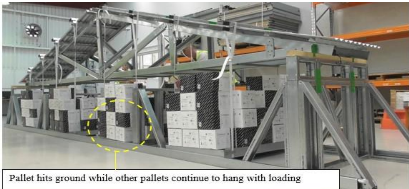
Figure 4-21: Pallet on ground at the end of Test 6
