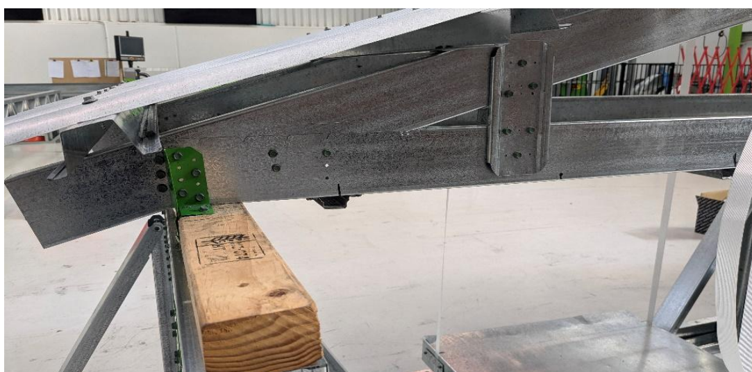
Figure 3-38: Example of 3 joints in the truss each with a minimum of 3 screws
