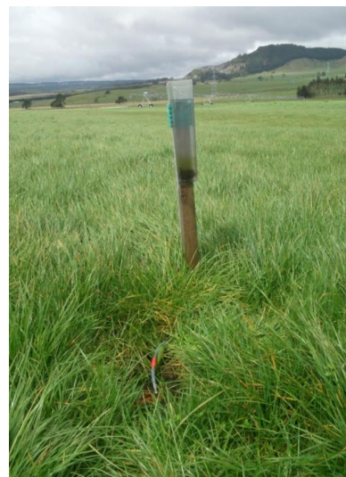
Figure 3.8. Lysimeter set up —plastic rain gauge, concrete pad, and sampling tube are visible.
