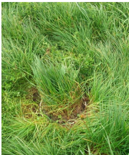
Figure 3.7. Lysimeter installed flush with the ground surface.
