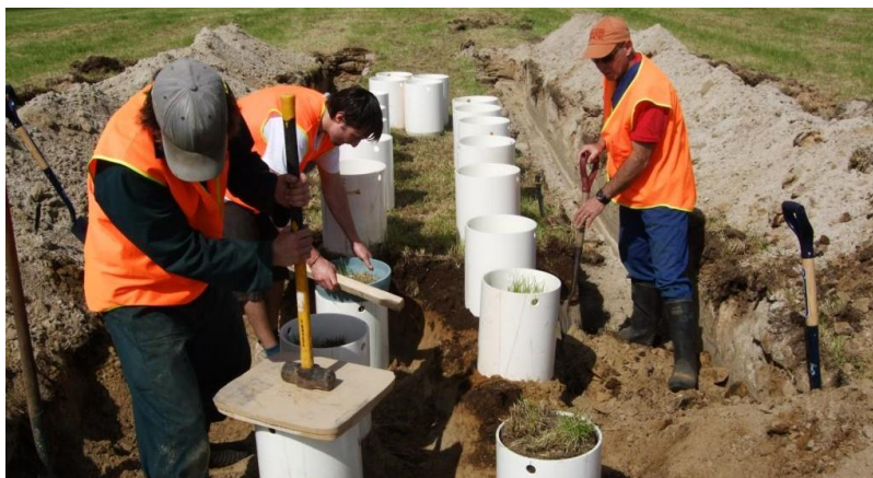
Figure 3.4. Construction of the barrel lysimeters. Photo, Glen TrewEEK.
