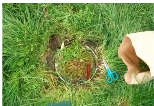
Figure 3.11. Grass cut to a height of 7 cm with scissors and collection into a paper bag.
