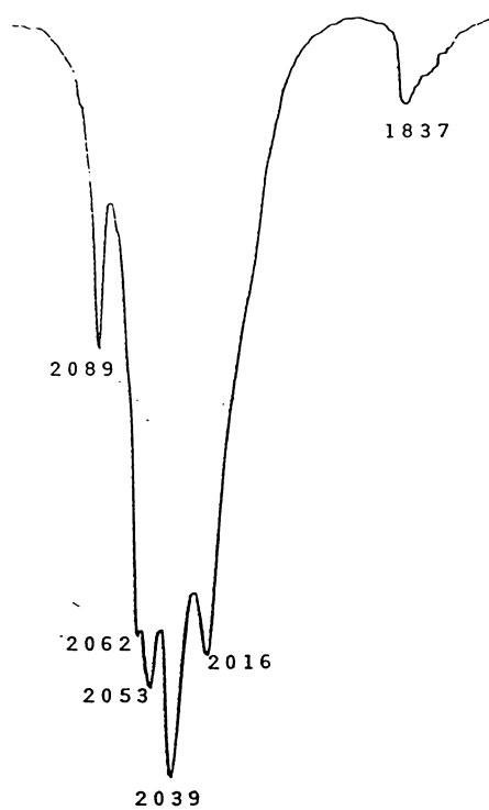
Fig 7.10 IR spcetrum of \text{Me}_2\text{Ge}_3\text{Co}_6(\text{CO})_{17} (in \text{CH}_2\text{Cl}_2 )
