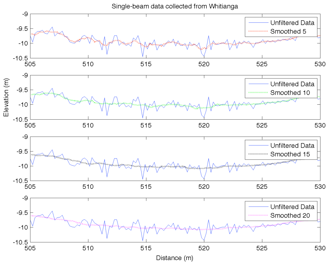
Figure 4.4: MATLAB figure showing the different levels of filtering applied to the raw data to filter out errors. Note the smoothed values are the number of values that the low pass filter uses to smooth the data.
