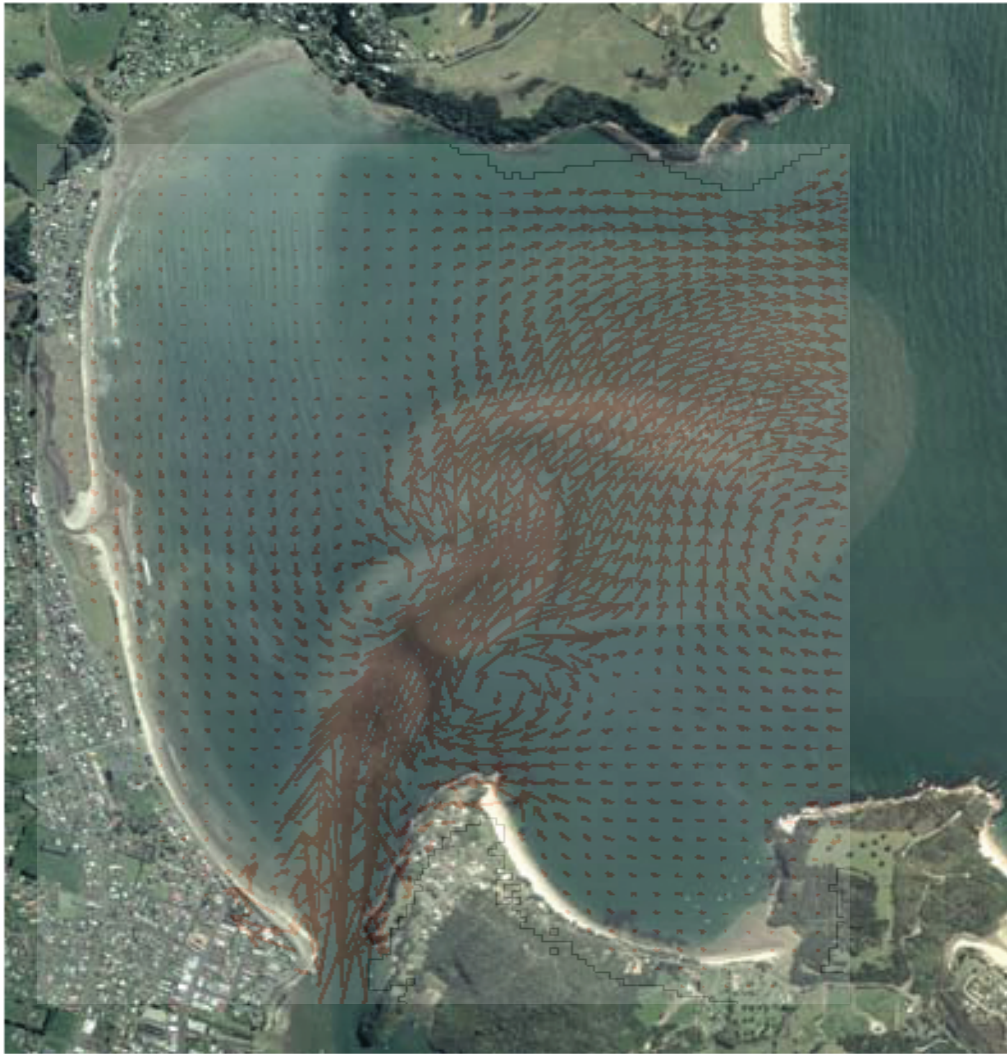
Figure A4: Ebb velocity vectors output by the 3DD model predicting an ebb tidal suspended sediment plume entering Mercury Bay.
