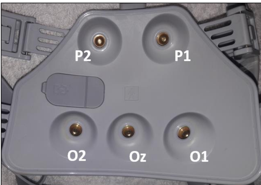
Figure 3.4: NuroChek electrode locations.
