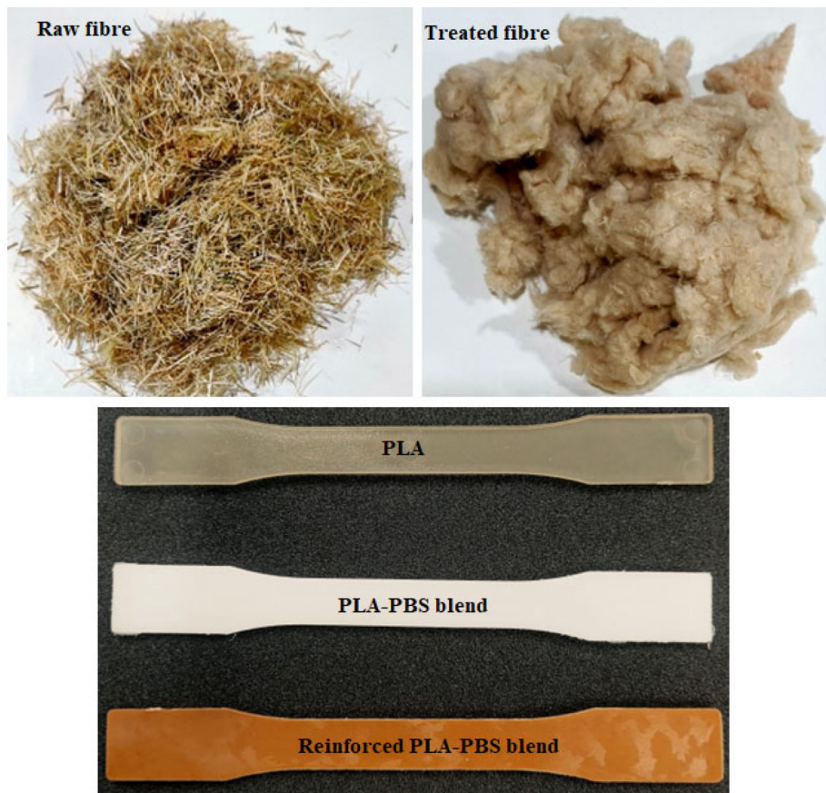
FIGURE 1 Digital images of raw harakeke fiber, treated (digested) harakeke fiber, and representative images of injection molded samples. PBS, polybutylene succinate; PLA, poly(lactic acid). [Color figure can be viewed at wileyonlinelibrary.com ]
