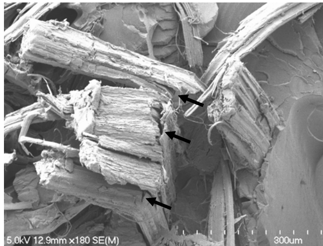
Figure 6.19: SEM micrograph for flexural tested fracture surface of UPE/FB2 composites showing kinks (indicated by arrows).
