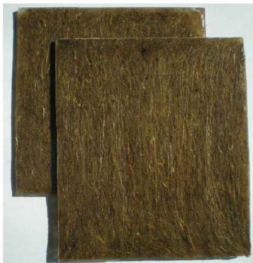
Figure 3.2: Aligned long hemp fibre reinforced PLA composites fabricated by compression moulding.
