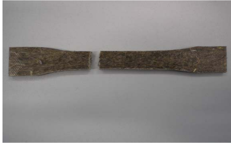
Figure 5.73: Photograph of a tensile tested aligned long hemp fibre (35 wt% fibre) reinforced PLA composite (PLA/ALK).
