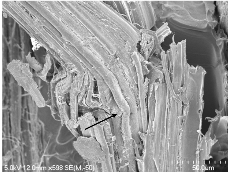
Figure 6.40: SEM micrograph of flexural tested long fibre composites (UPE/ALKSIL) showing kinks (indicated by arrow).
