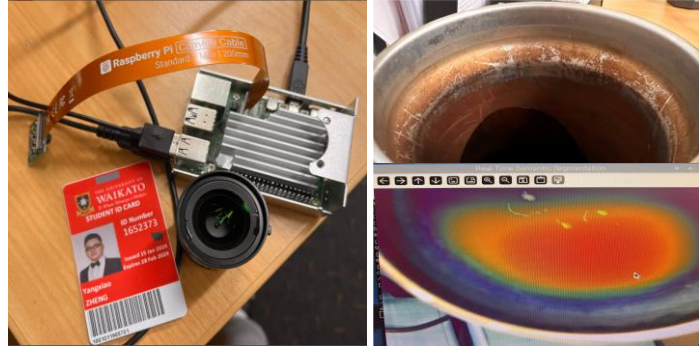
Fig. 13. Real-world deployment of Bayesian-U 2 -Net on Raspberry Pi 4 with Camera Module V3 and custom lens, enabling real-time corrosion capture and onboard inference.
