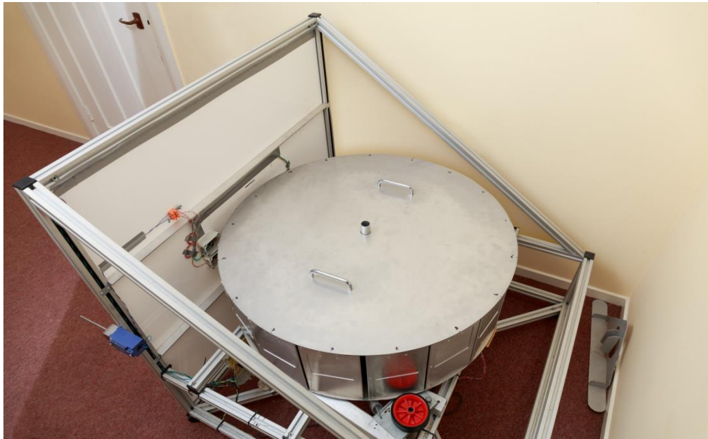
Figure 2. Scent-detection apparatus with the lid positioned on top of the segments.
