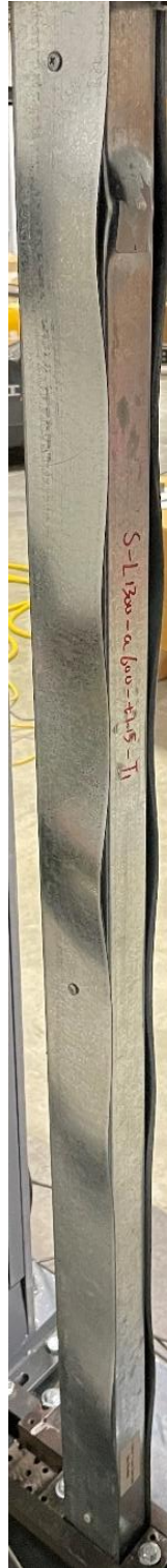
Figure 5-18 Failure progression of specimen SC-L1300-a600-t1.15-W1
