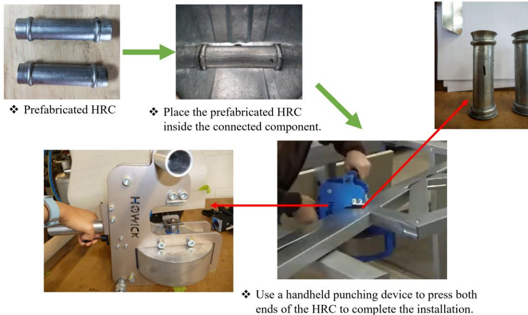
Figure 2-7 HRC installation process
