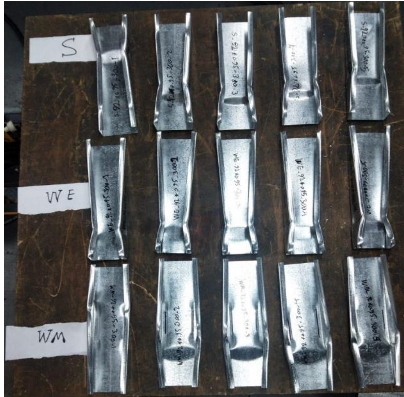
Figure 7-12 Failure modes of column having the cross-section of 92.1×42.3×0.95 mm
