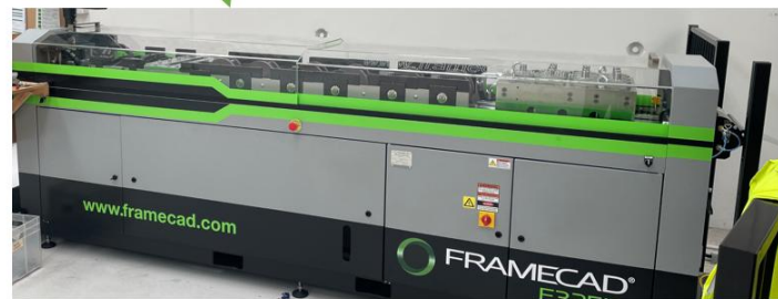
❖ Roller-forming, cutting, and pre-punching
