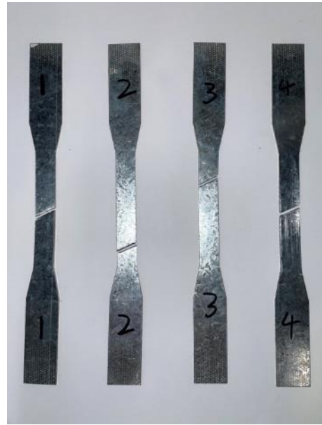
Figure 6-6 Deformed tensile coupons for G500 specimens
