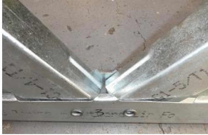
(b) Photograph of a field test Figure 4-3 Web member having swaged sections
