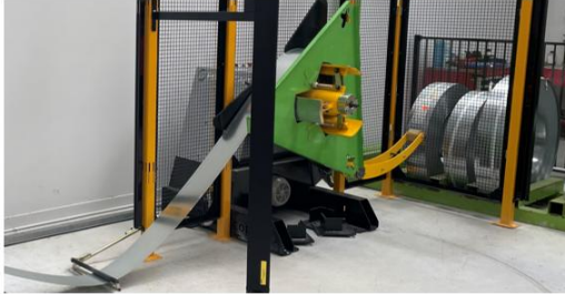
❖ Steel sheet coil-uncoiling and flattening
