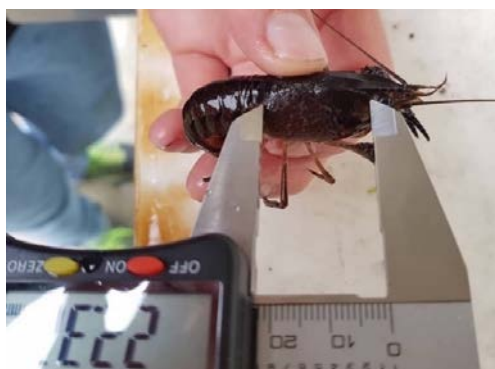
Figure 3-6. Measuring kōura orbital-carapace length (OCL) using digital callipers (Photo: A. Pearson, University of Waikato).
