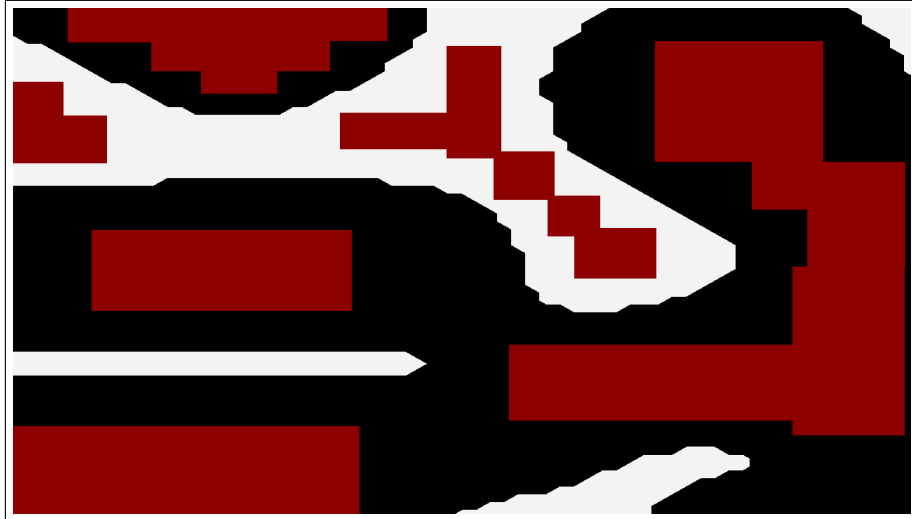
Figure 3.3: 2D Marching Squares example with red highlighted regions noting general areas which could be culled.
