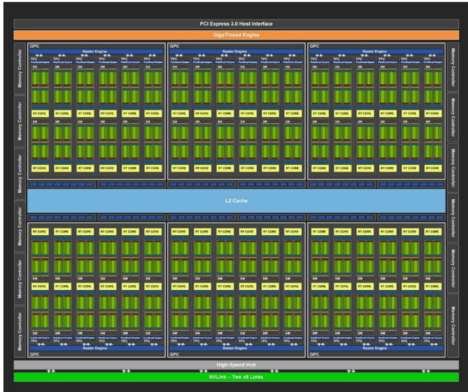
Figure 2.6: Turing TU102 Full GPU with 72 SM Units. Reproduced from Kilgariff et al. (2018).
