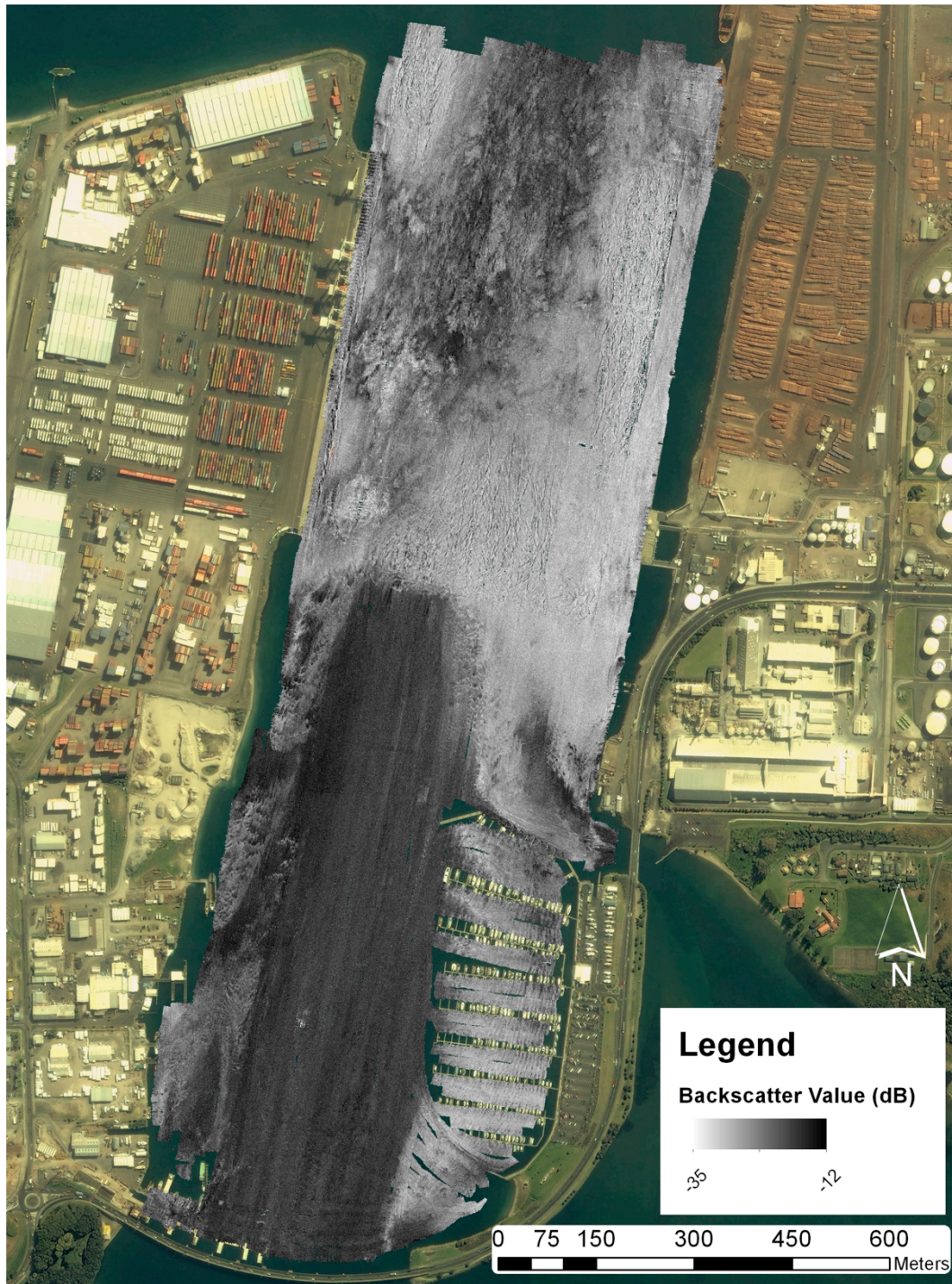
Figure 5.25: Multibeam echosounder backscatter mosaic of the Tauranga Harbour, based on the survey performed in August 2011.
