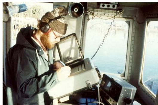
Figure 2.15: Single-beam echosounder recording onboard the BOPHB work vessel "Mahi". (Source: de Lange, 2011)
