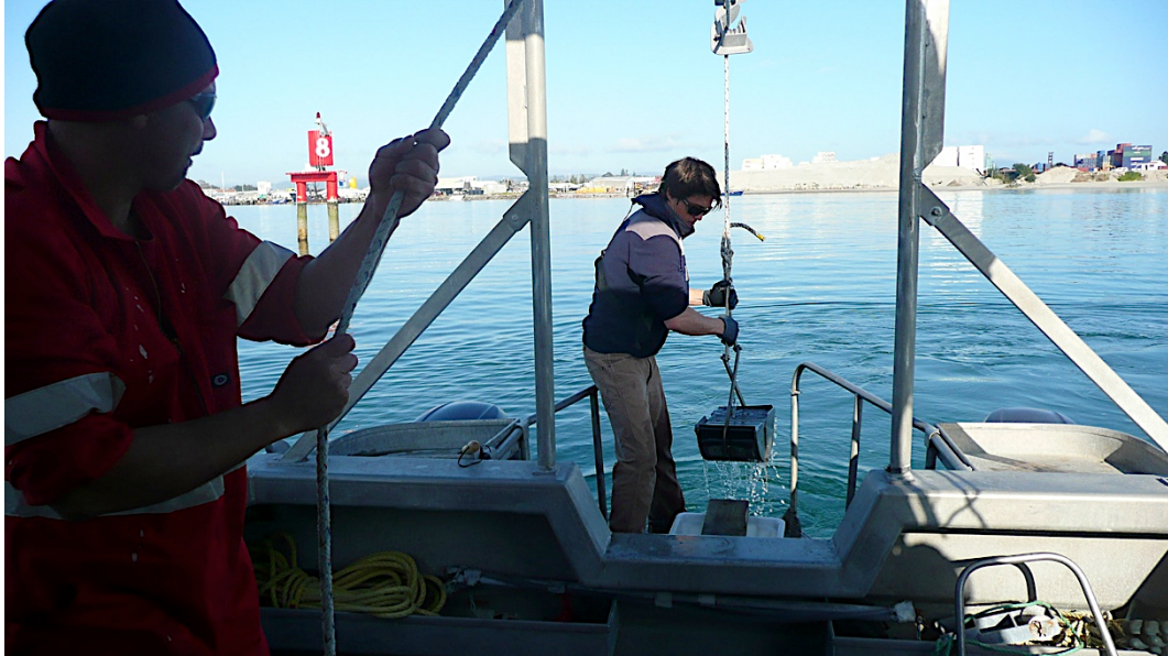
Figure 4.2: Sediment sampling setup on the University of Waikato's survey vessel Tai Rangahau . The capstan hauling the Ponar grab sampler through the pulley on the davit (visible on top) is located on the left behind the operator.
