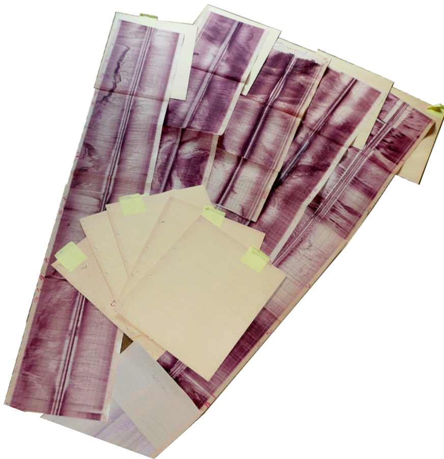
Figure 6.2: Sidescan sonar paper recordings of the Tauranga Harbour Study (Healy, 1985)
