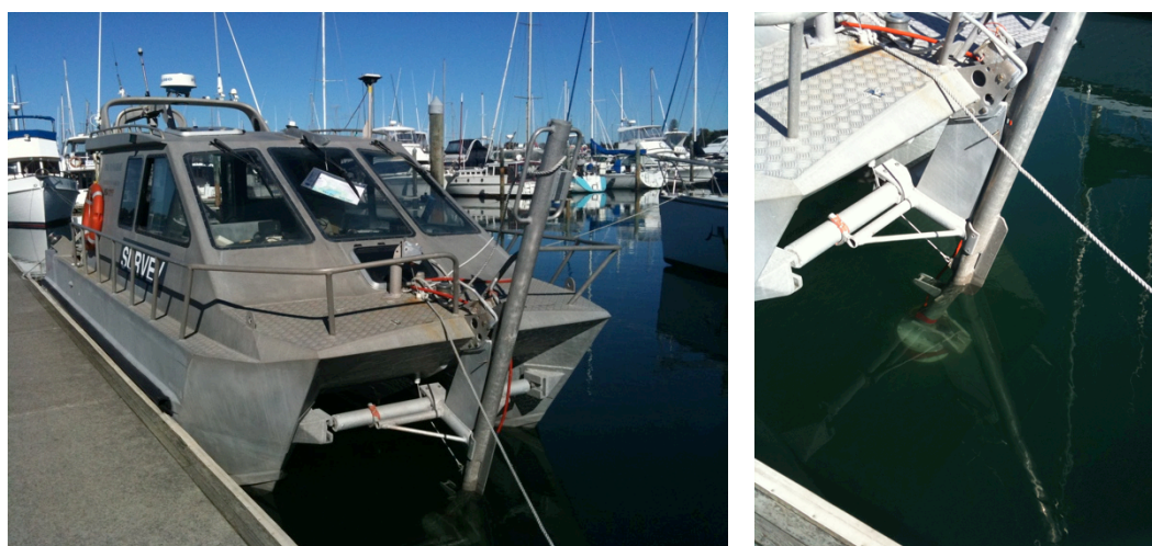
Figures 5.13 & 5.14: University of Waikato survey vessel Tai Rangahau (left) showing the Kongsberg EM3000 fitted on a bow pole (right).
