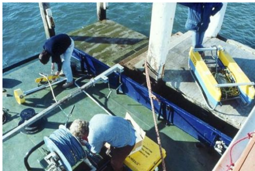
Figure 2.14: Klein sidescan sonar system (towfish) and Uniboom Seismic profiler. (Source: de Lange, 2011)
