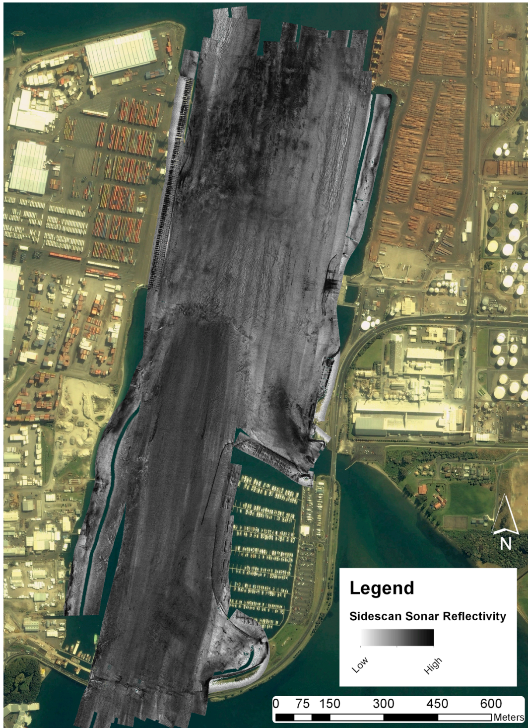
Figure 5.6: Sidescan sonar reflectivity mosaic of the Port of Tauranga (July 2011).
