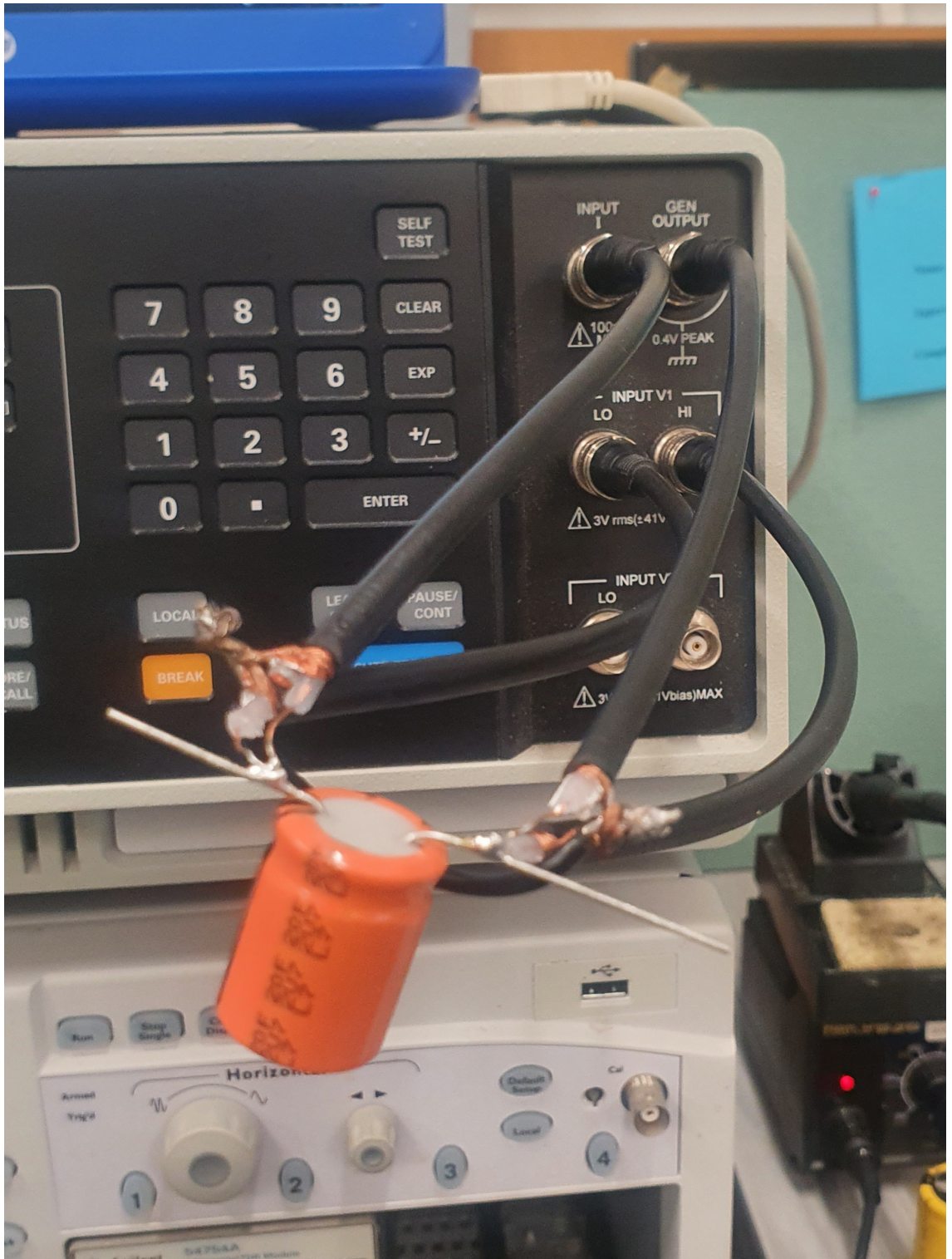
Figure 5.1: Device under test connected to the Solartron 1260A in the 4-wire arrangement.
