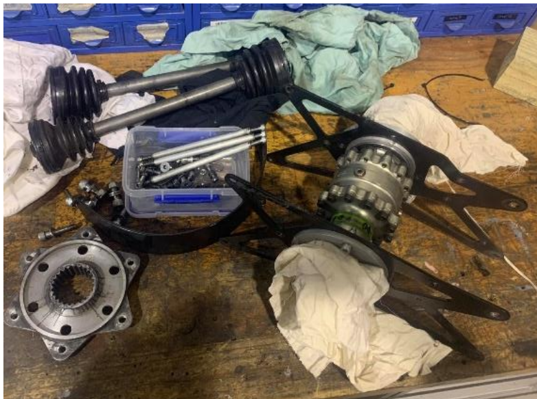
Figure 38: W-FS-18 Drivetrain components
