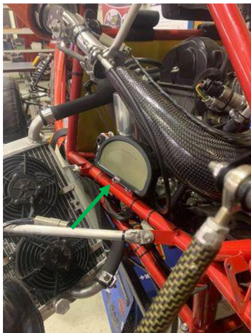
Figure 43: MoTeC unit mounting location
