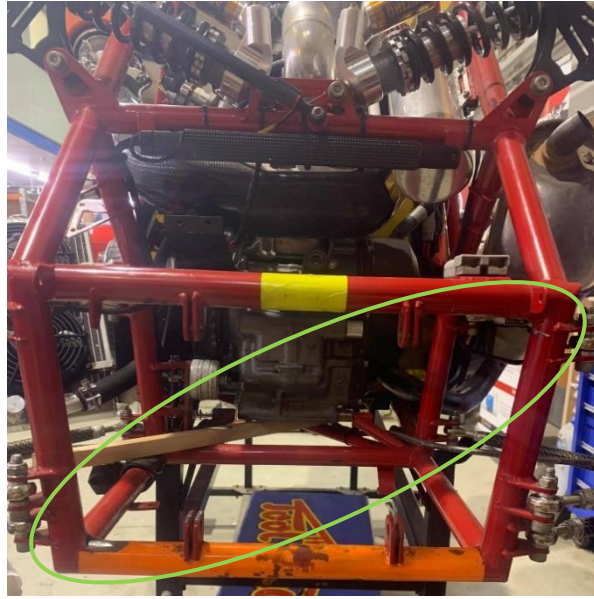
Figure 47: W-FS-18 chassis with rear cross brace removed
