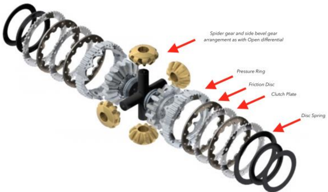
Figure 26: Exploded view of Drexler 2010 FSAE Limited Slip Differential
