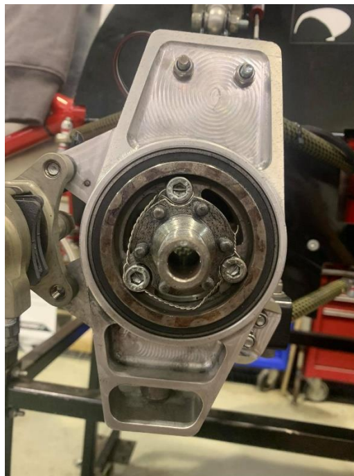
Figure 88: Hub assembly with safety locking wire for bolts holding the hub together
