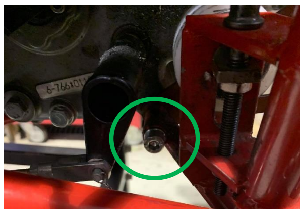
Figure 93: Engine bolt that fell out
