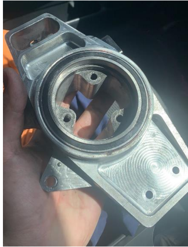
Figure 87: Upright with disassembled hub after bearing replacement
