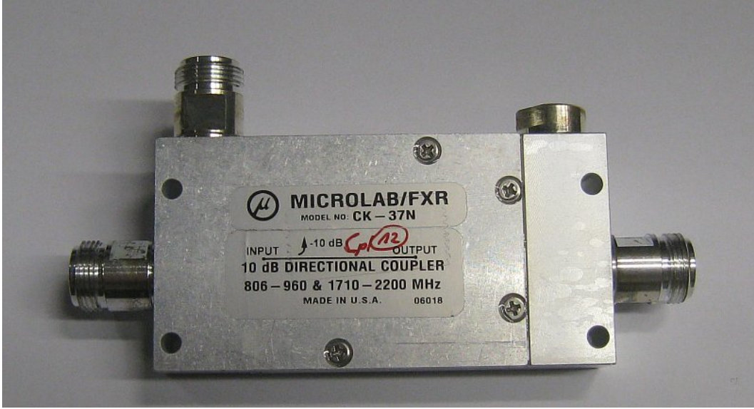
Figure 2.2: An example of a 10 dB 1.7--2.2 GHz directional coupler with N-type coaxial connections. Ports from left to right: input, coupled, isolated (terminated internally), and the transmitted port. Image credit: Vonvon CC BY-SA 3.0
