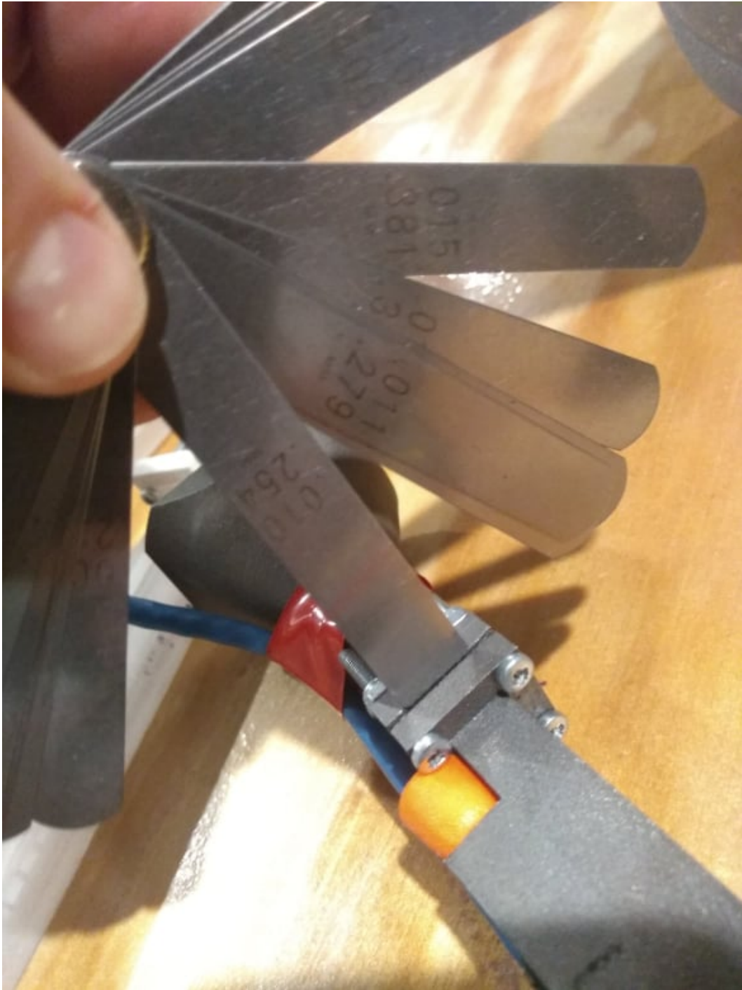
Figure 3.21: An imperial (Thou/mm) feeler gauge inserted between two 3D printed titanium (Ti64) flanges bolted up to their rated torque. The gap is approx 10 Thou or 0.254 mm.
