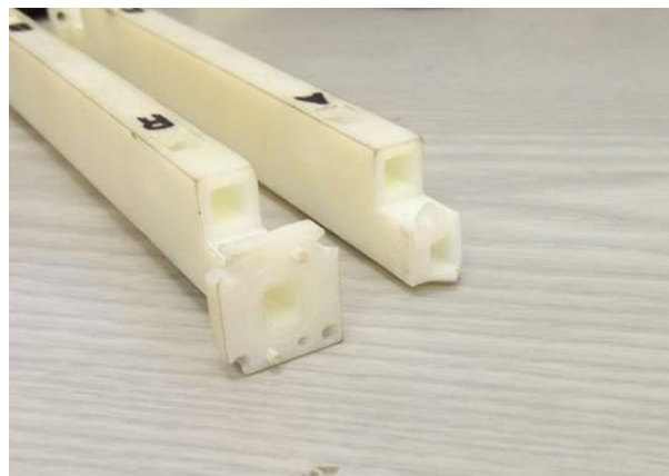
Fig. 3. Examples of broken flanges from repeated use without U-shaped washers.
