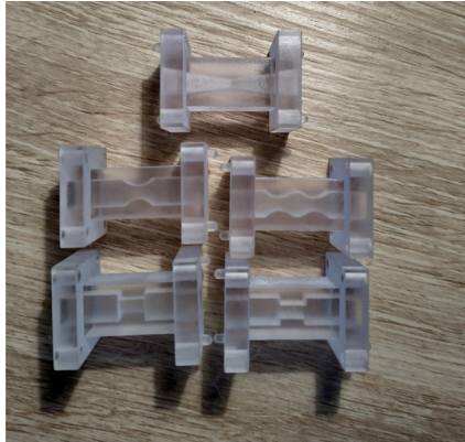
Figure 6.1: A selection of transmission lines, of varying geometry designed for the 10–20 kHz bandwidth.
