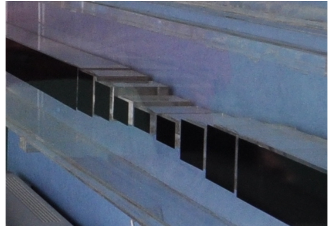
Fig. 6. A Lagasse coupler constructed in transparent acrylic with black tape marking the divide between parallel waveguides and the branch-line section.
