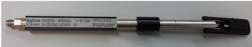
Figure 2.16: An example of a sliding load from Agilent technologies, 00915-60004 2.4mm sliding load. Image credit: A13ean. This file is licensed under the Creative Commons Attribution-Share Alike 3.0 Unported license. https://creativecommons.org/licenses/by-sa/3.0/deed.en
