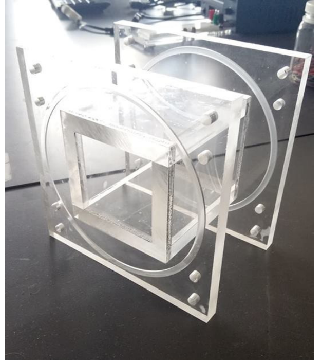
Fig. 8. Photograph of a short thru in the low-frequency, acrylic waveguide.
