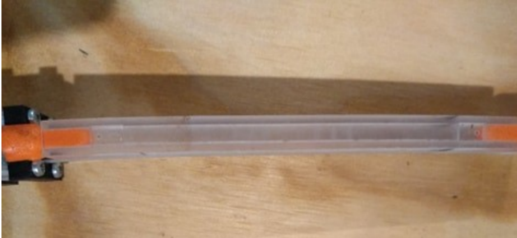
Figure 3.16: The warping (in the plane of the image) of the length of the directional coupler is visible. Two red straight lines have been added to help show the warping.
